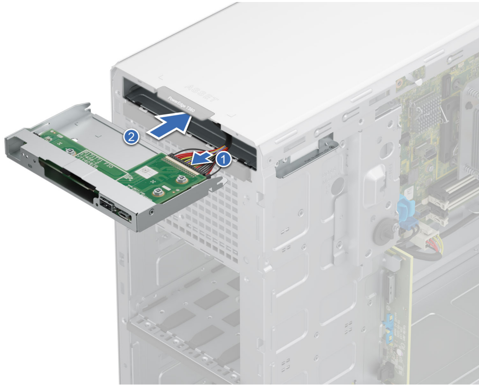
Figure 96. Installing the control panel cage
