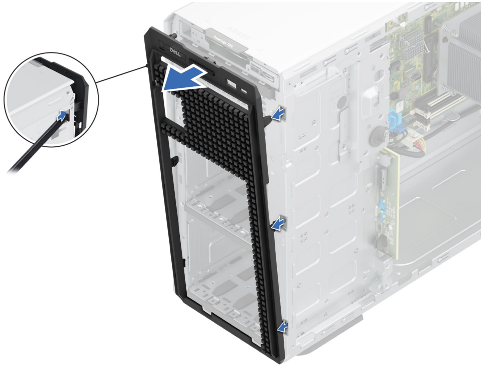
Figure 92. Removing the front faceplate
