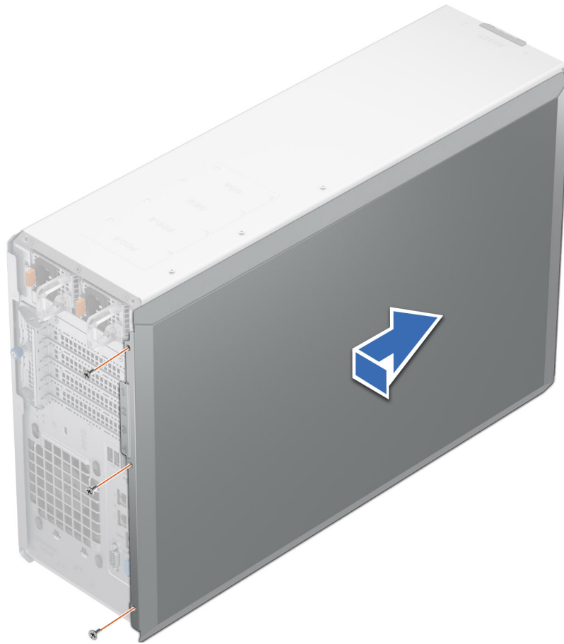
Figure 98. Installing the system side cover
