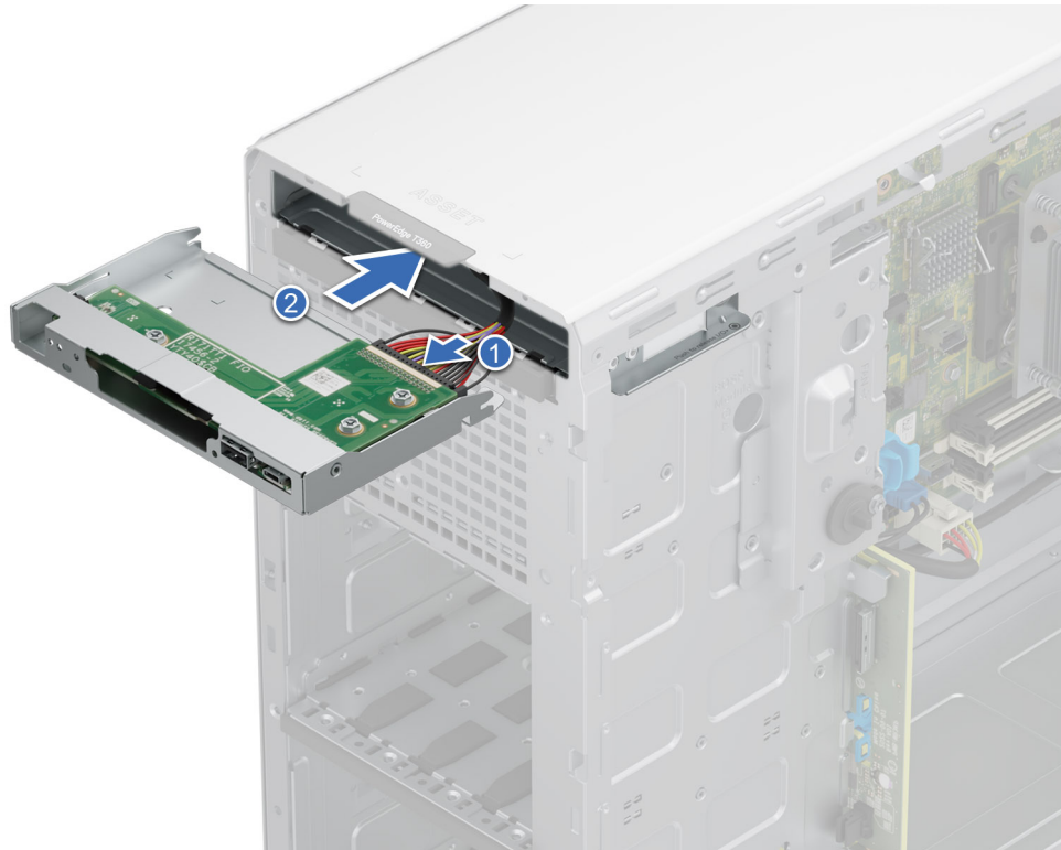
Figure 96. Installing the control panel cage
