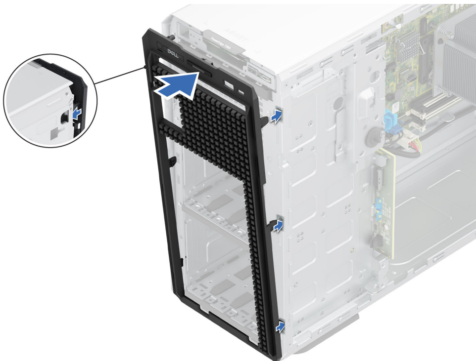
Figure 97. Installing the front faceplate
