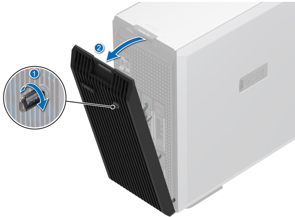
Figure 12. Removing the front bezel
