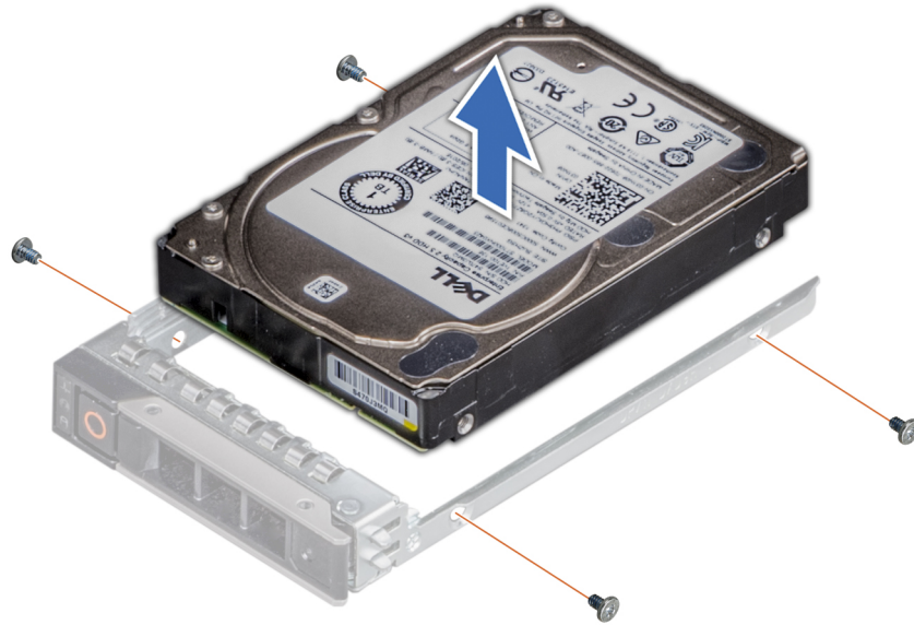
Figure 28. Removing the drive from the drive carrier
