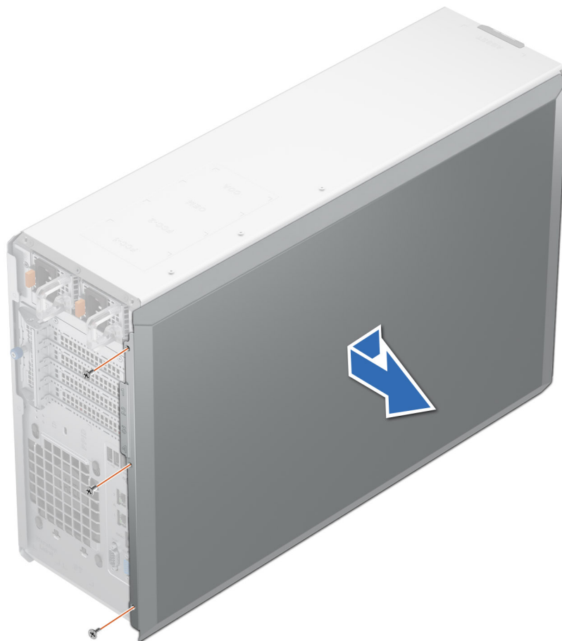
Figure 91. Removing the system side cover
