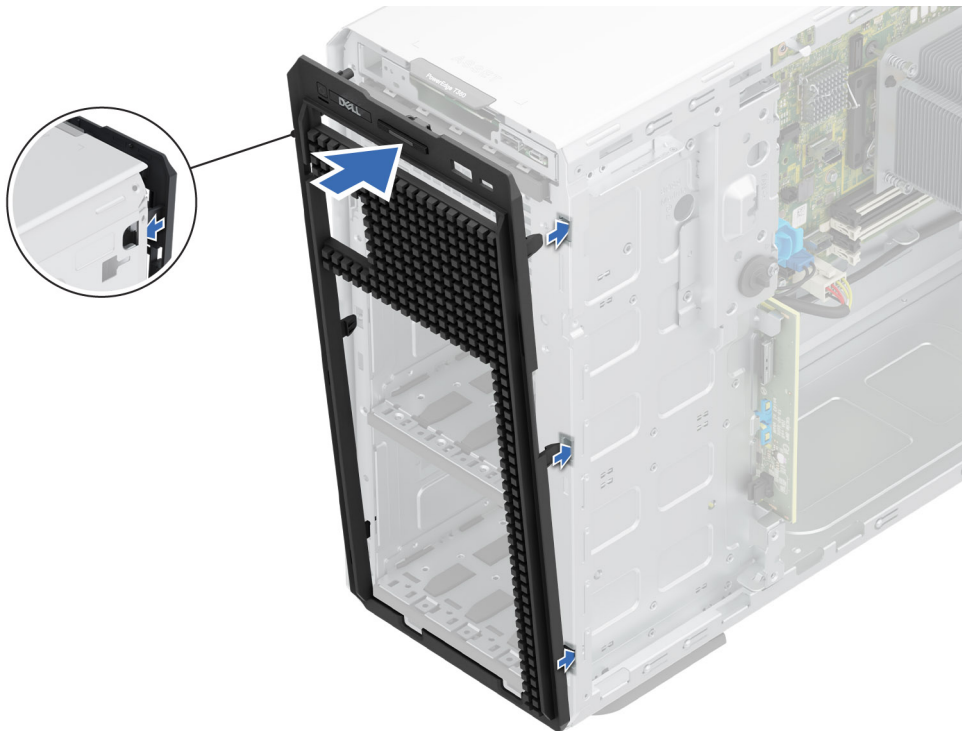
Figure 97. Installing the front faceplate
