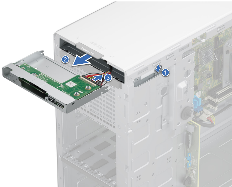
Figure 93. Removing the control panel cage
