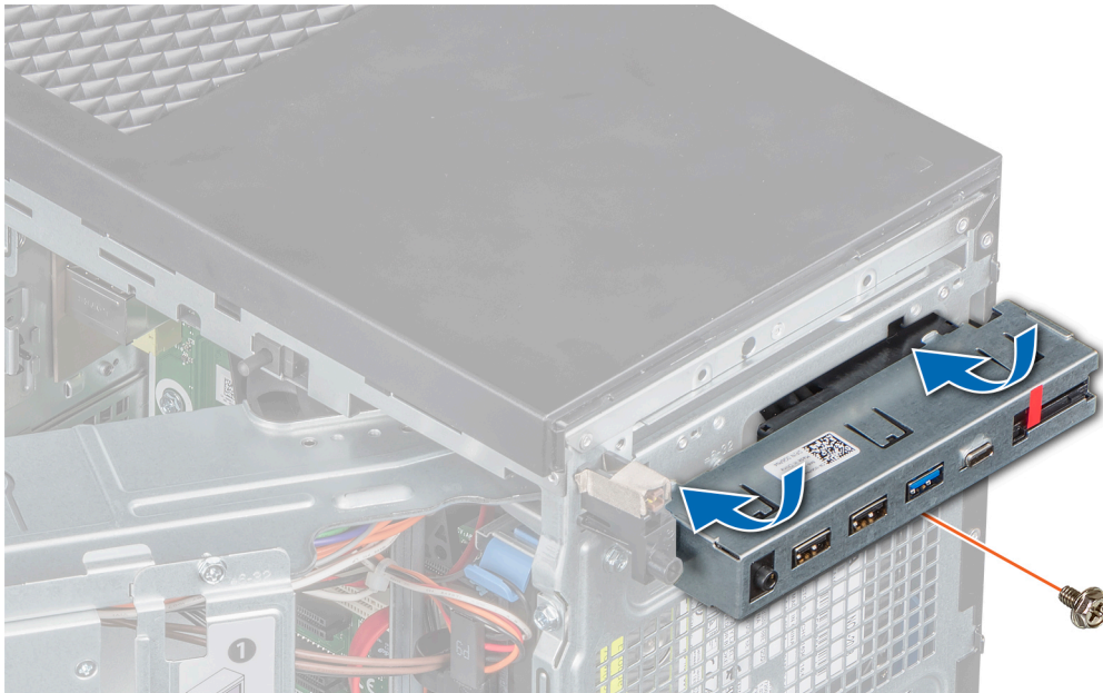
Figure 53. Installing the control panel
