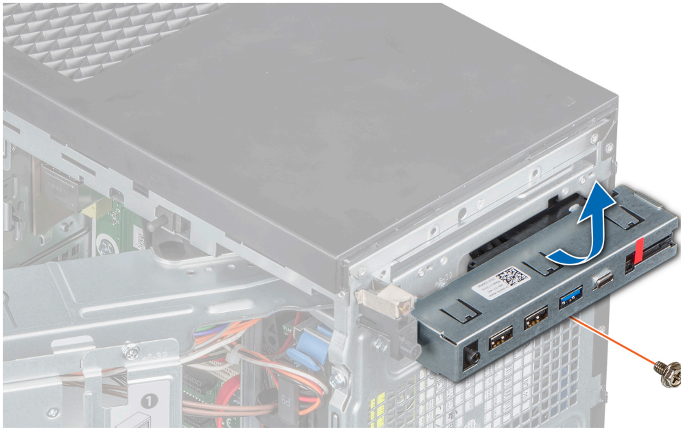
Figure 52. Removal of the control panel
