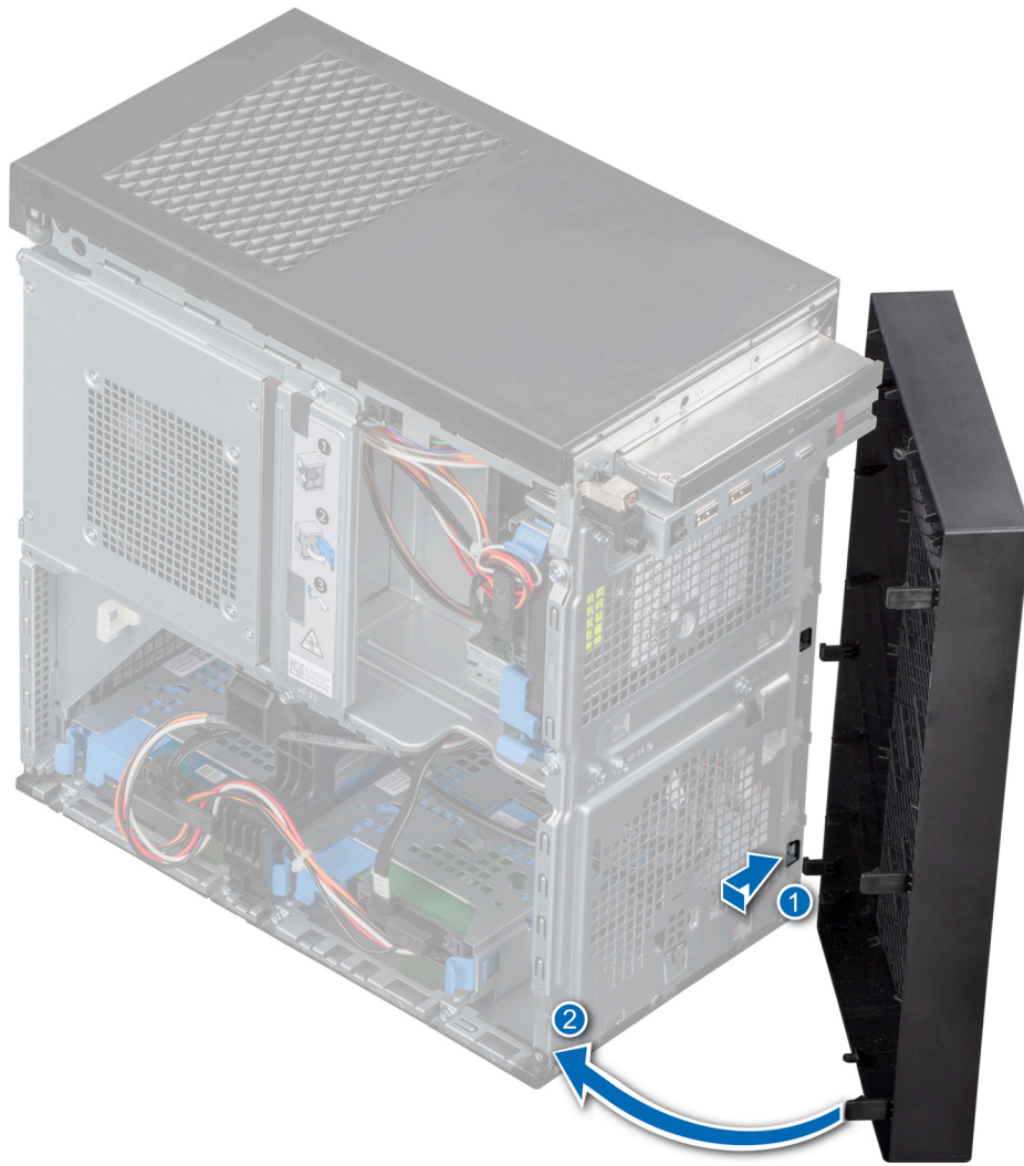
Figure 13. Installing the front bezel
