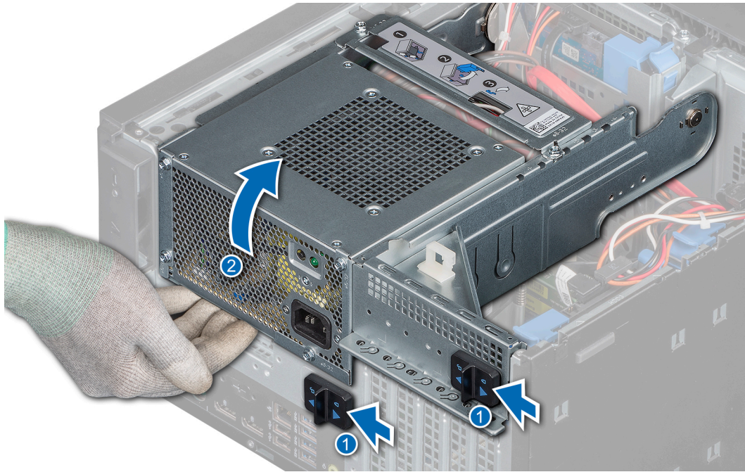
Figure 18. Opening the PSU assembly
