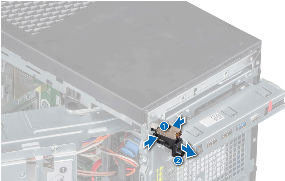
Figure 54. Removing the power button module
