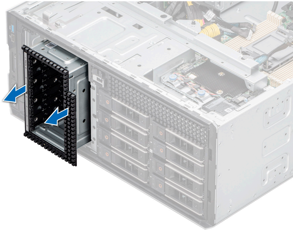
Figure 68. Removing a NVMe drive bay
