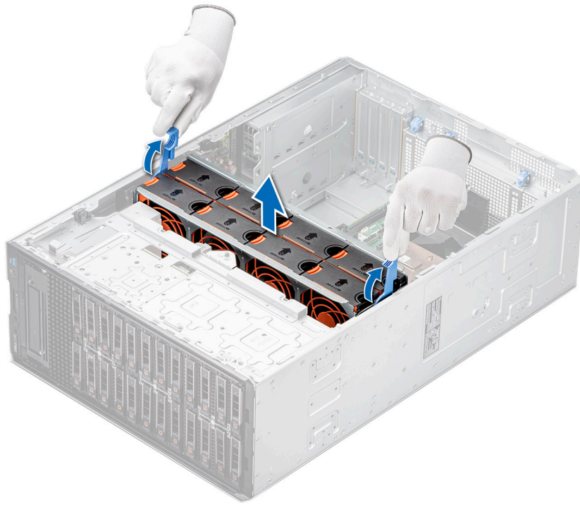
Figure 37. Removing the cooling fan cage
