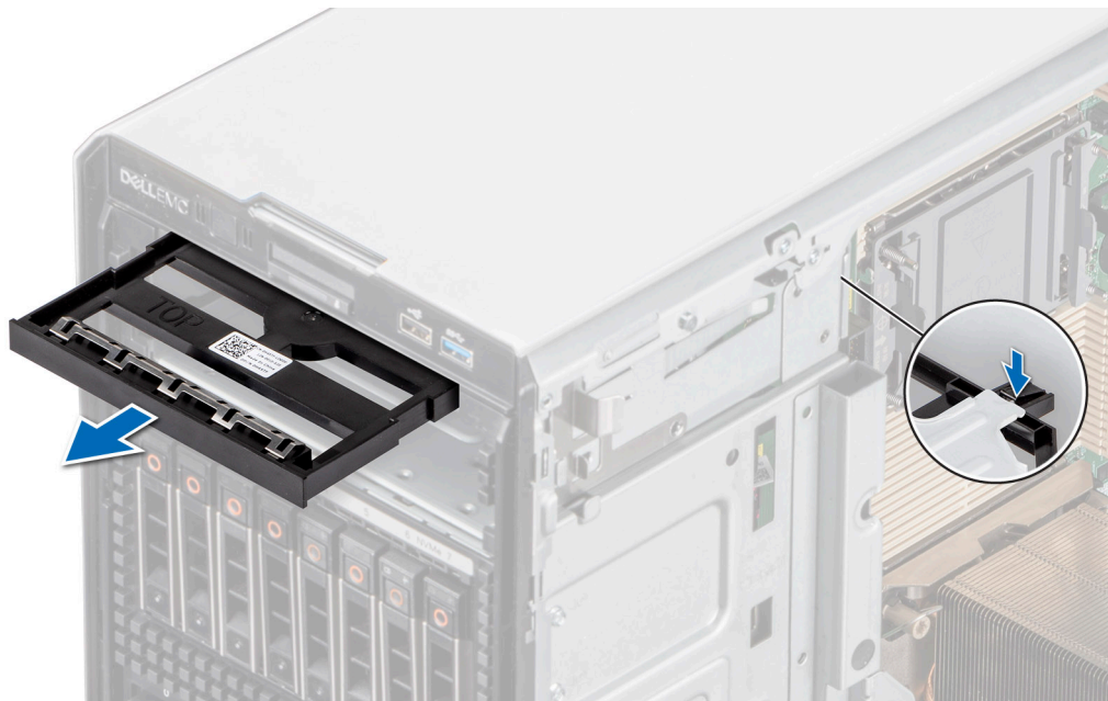
Figure 93. Removing the optical drive blank
