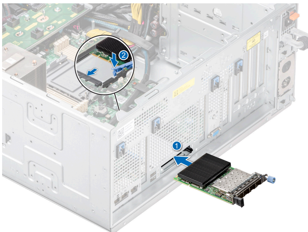
Figure 155. Installing the OCP card
