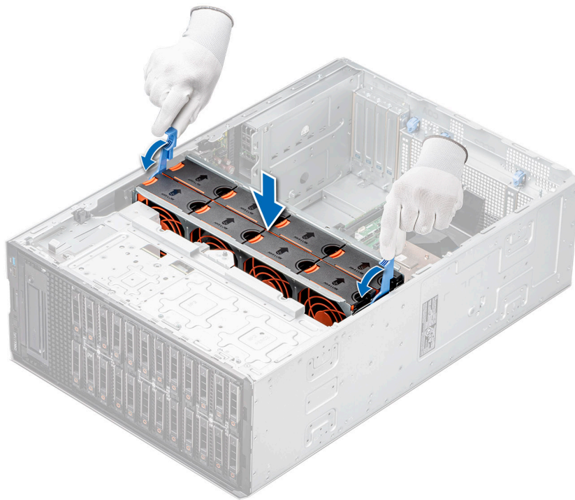
Figure 38. Installing the cooling fan cage
