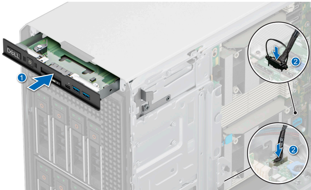
Figure 134. Installing the front IO module
