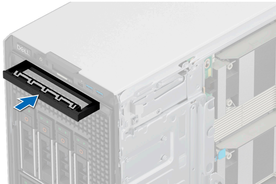
Figure 126. Installing the optical drive blank
