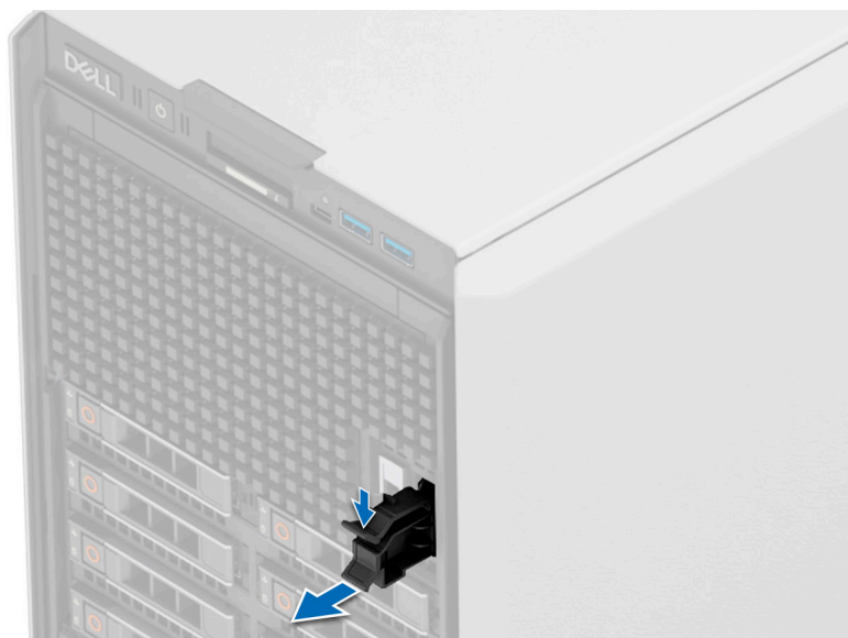
Figure 145. Removing the BOSS-N1 card carrier blank
