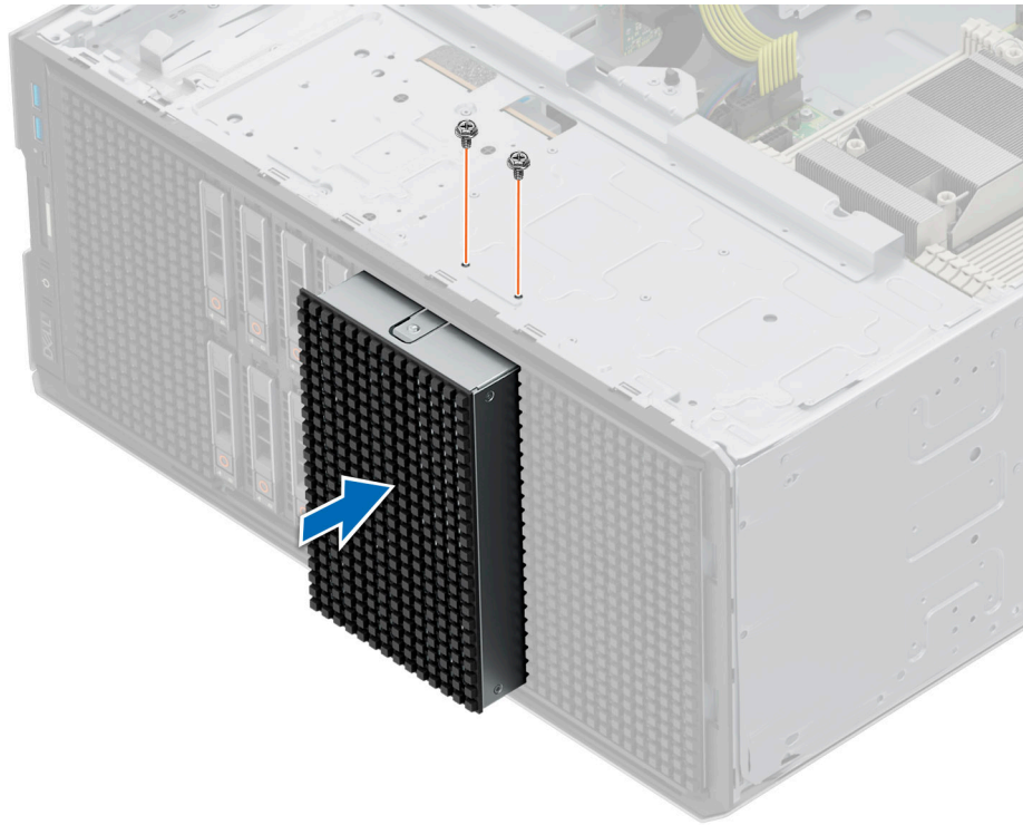
Figure 116. Installing the drive bay blank
