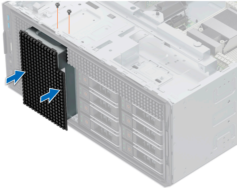
Figure 118. Installing the NVMe drive bay blank
