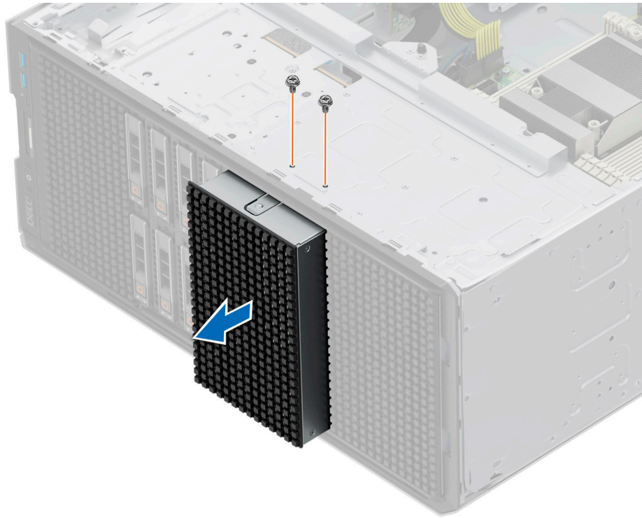
Figure 113. Removing the drive bay blank
