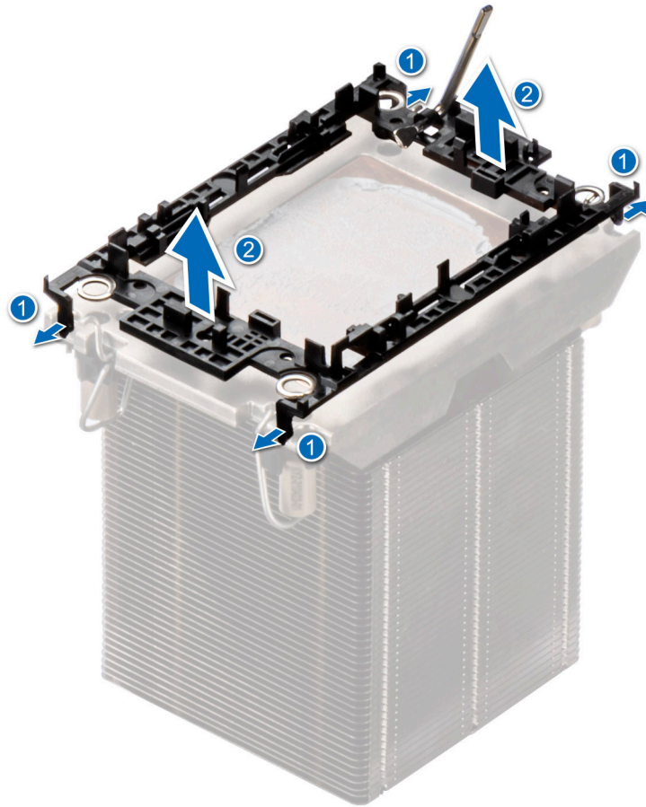
Figure 164. Removing the retaining clip
