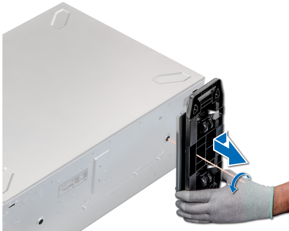
Figure 25. Removing caster wheels
