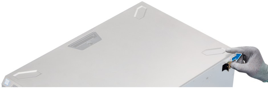
Figure 115. Attaching the mylar cover
