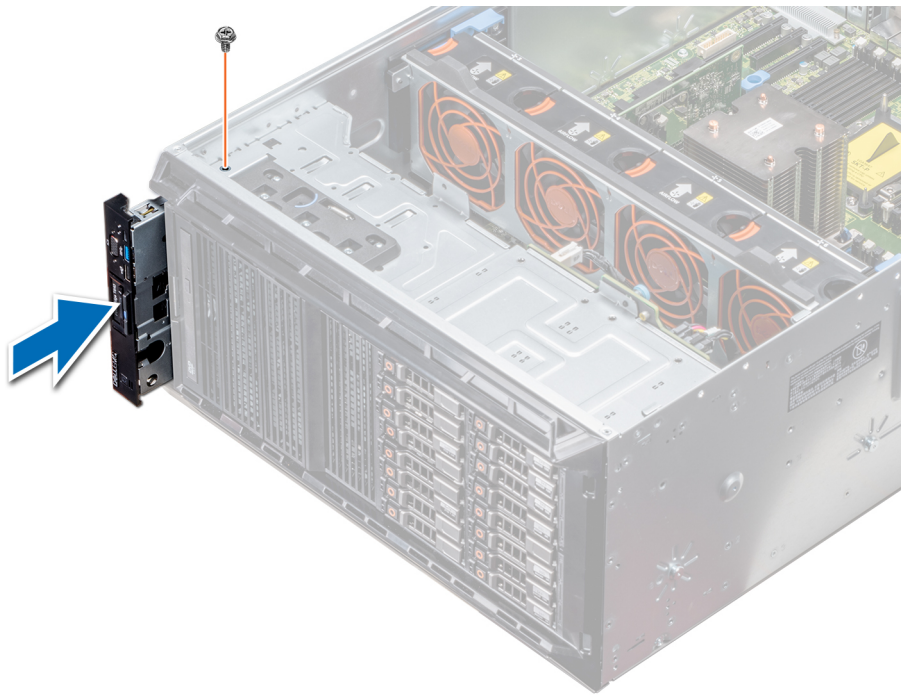
Figure 103. Installing the control panel assembly
