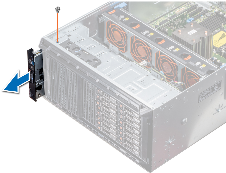
Figure 100. Removing the control panel assembly
