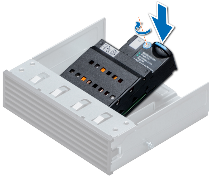
Figure 66. Installing the NVDIMM-N battery
