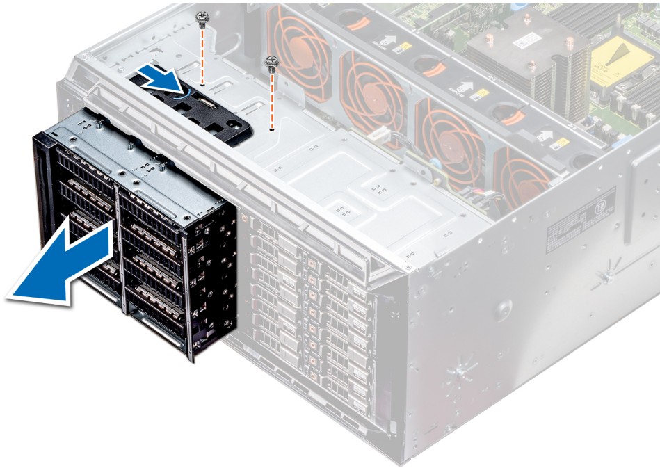
Figure 57. Removing a NVMe drive bay or flex bay
