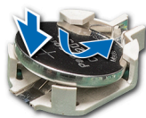
Figure 105. Installing the system battery
