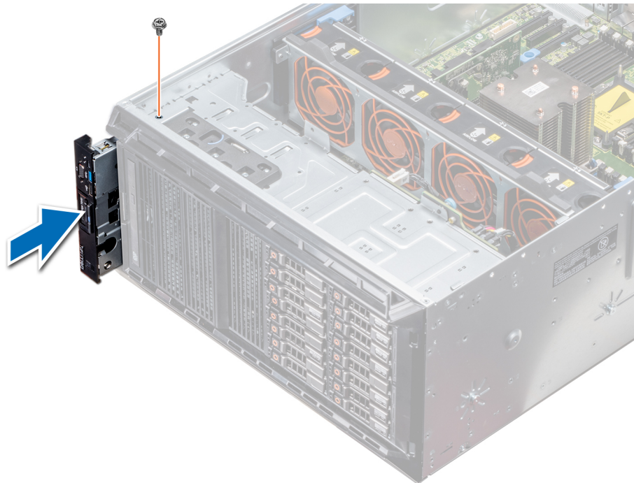
Figure 109. Installing the control panel assembly
