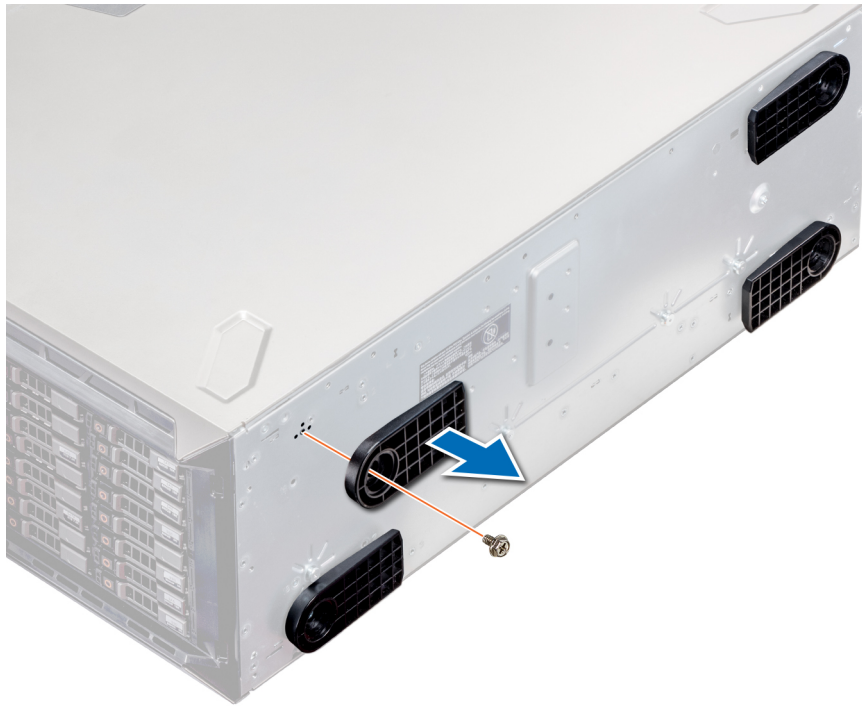
Figure 27. Removing the system feet
