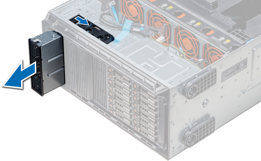
Figure 59. Removing the optical drive or tape drive
