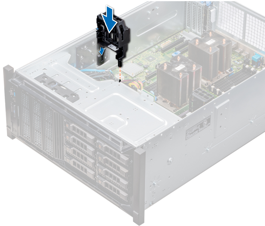
Figure 80. Installing the optional GPU card holder
