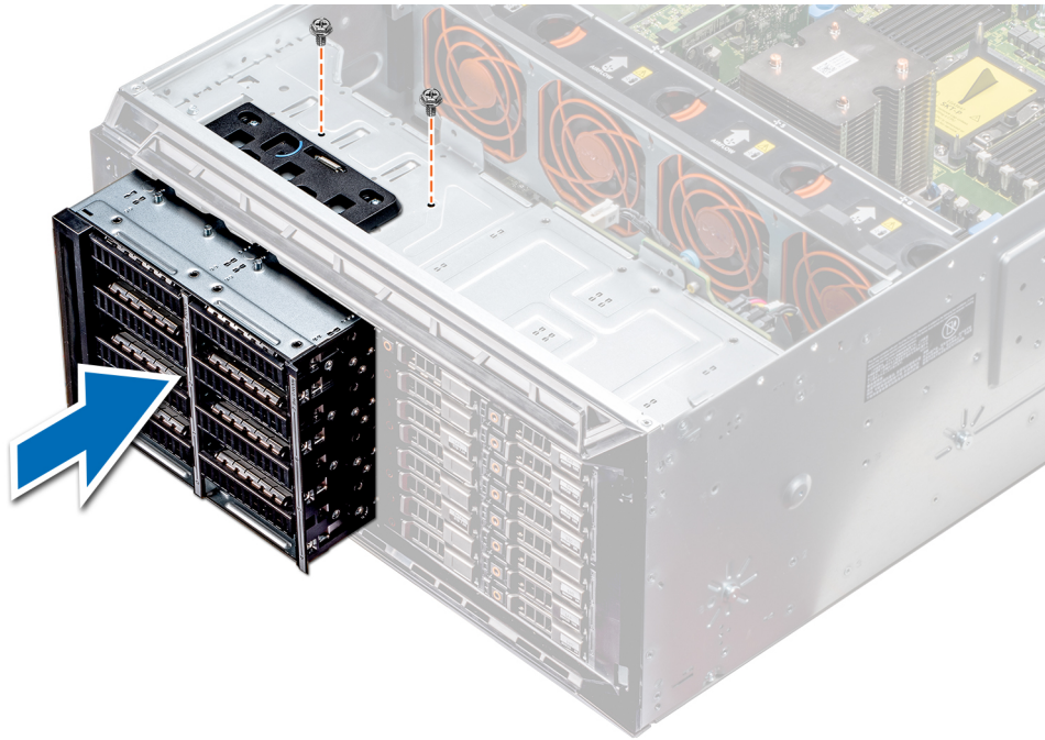
Figure 58. Installing a NVMe drive bay or flex bay
