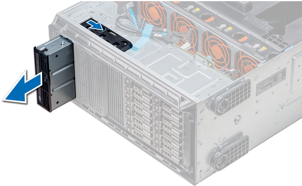
Figure 61. Removing the optical drive cage or tape drive
