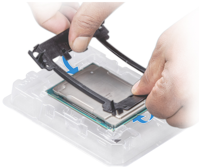
Figure 73. Installing the processor bracket
