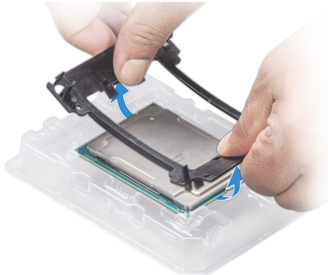
Figure 72. Removing the processor bracket
