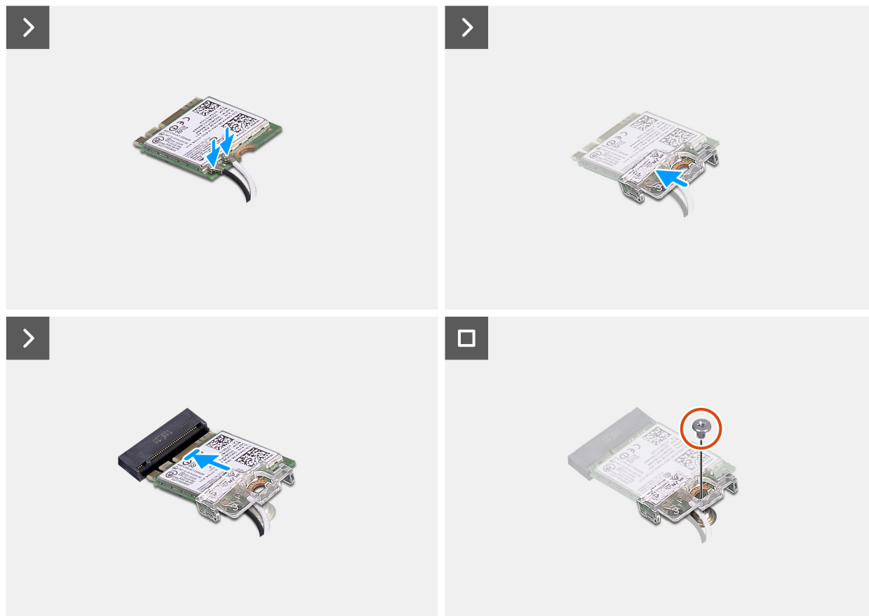
Figure 27. Installing the WLAN card
