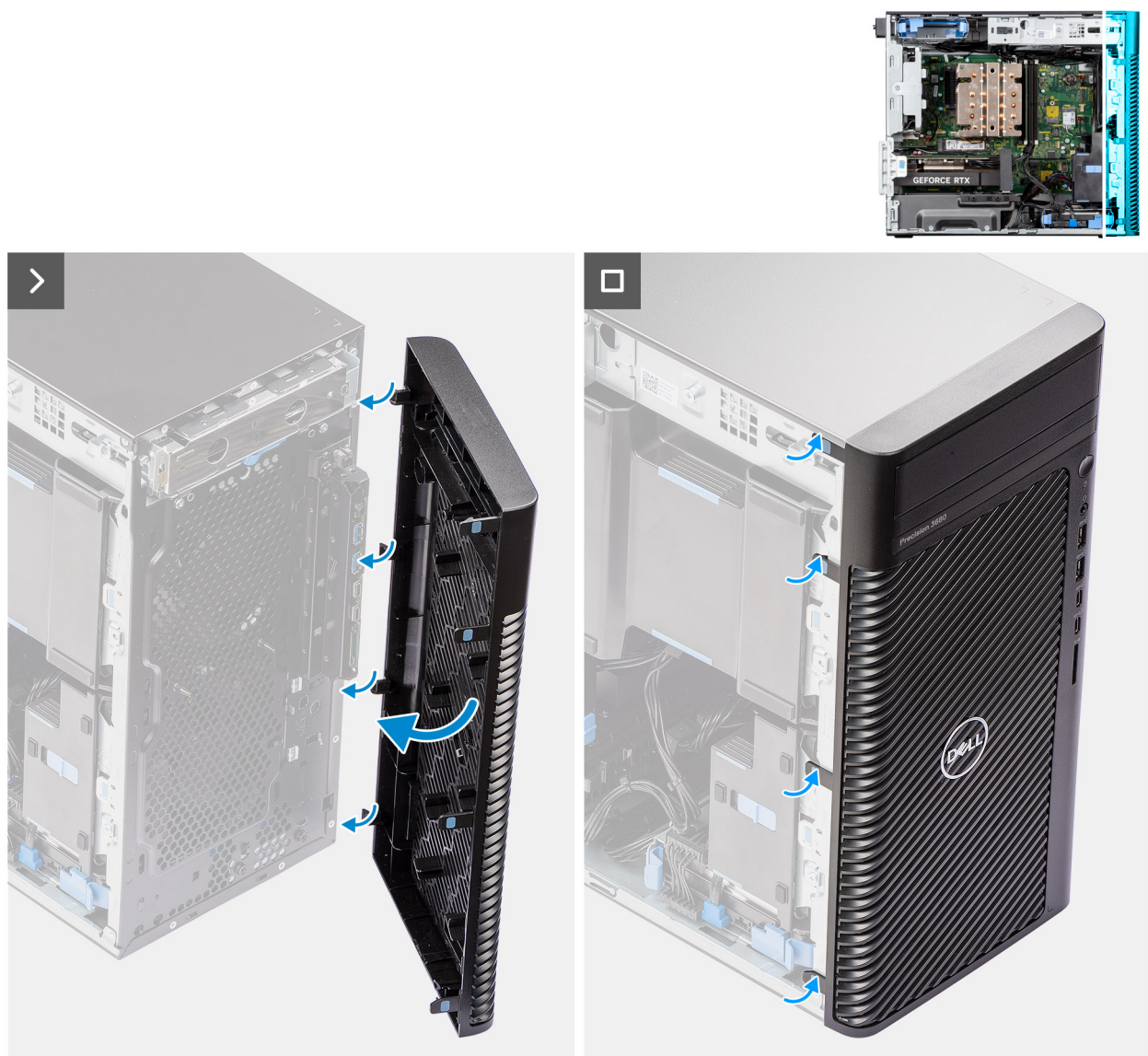
Figure 13. Installing the front bezel
