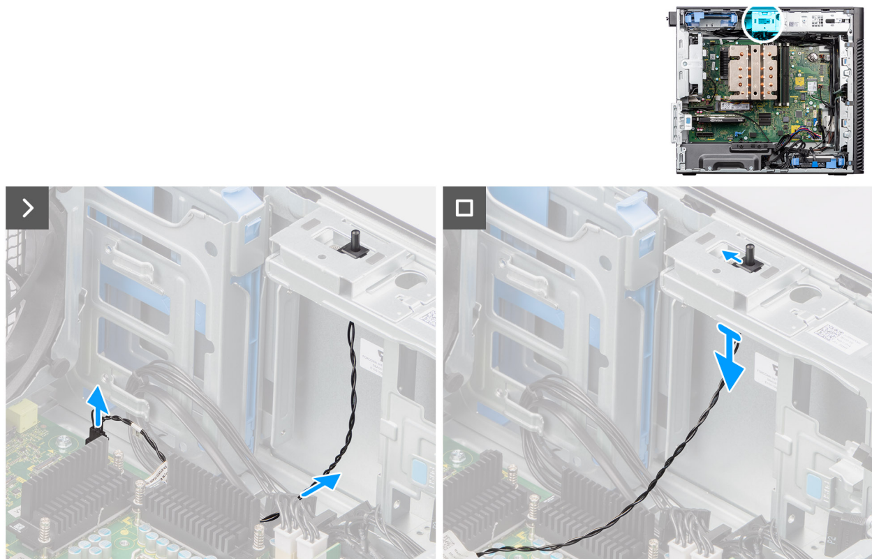
Figure 70. Removing the intrusion switch
