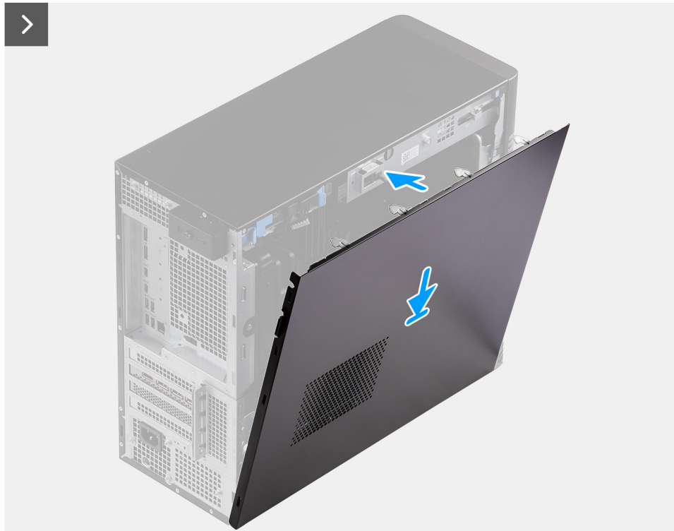
Figure 10. Installing the side cover
