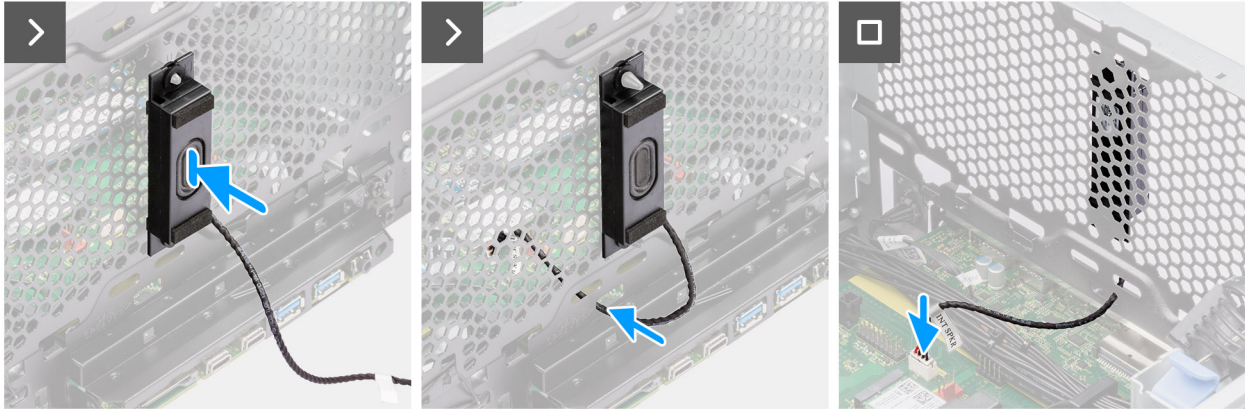
Figure 73. Installing the internal speaker
