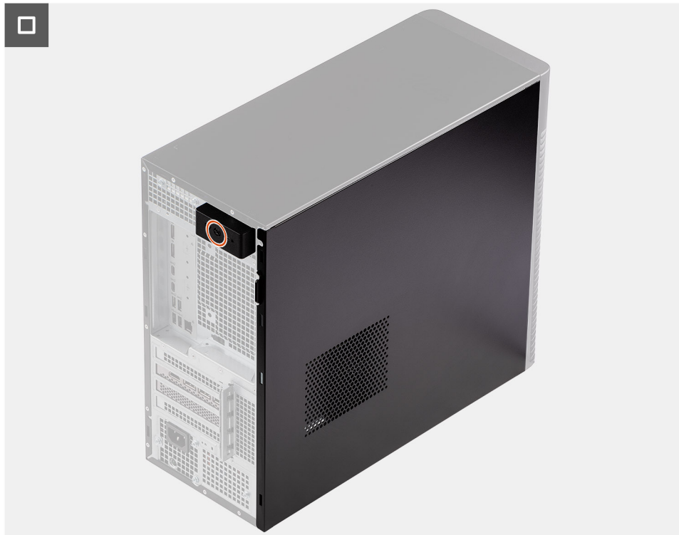
Figure 11. Installing the side cover
