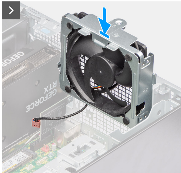
Figure 67. Installing the rear fan (1000W PSU)
