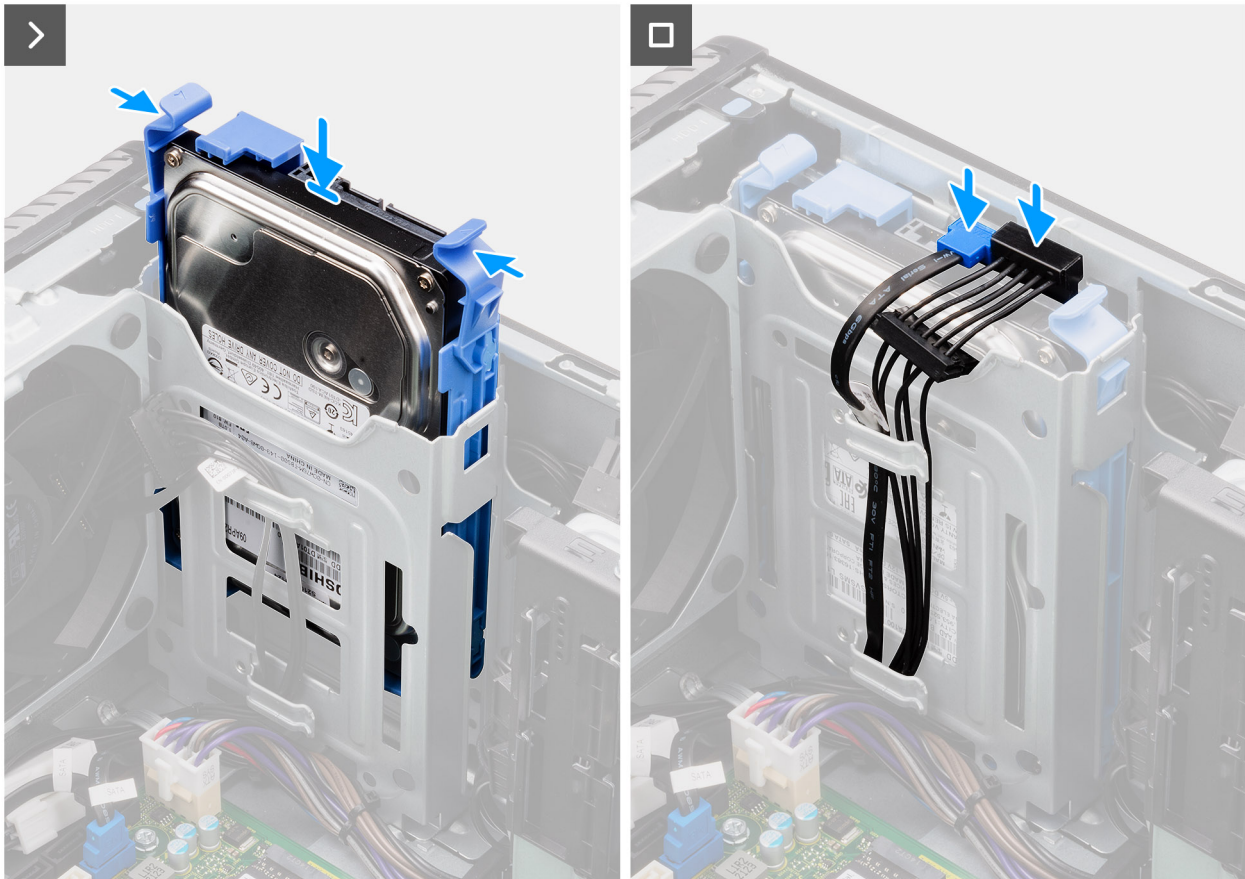
Figure 20. Installing the 3.5-inch hard drive assembly (Bay-2)
