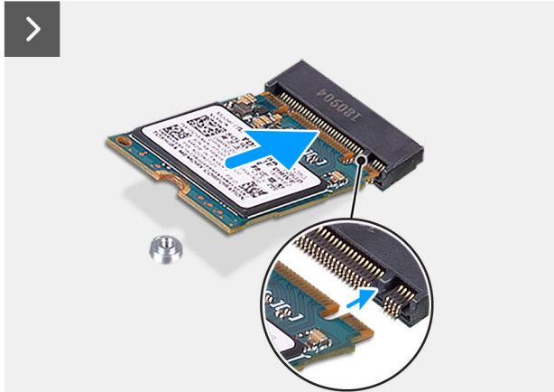
Figure 23. Installing the M.2 2230 PCIe solid state drive
