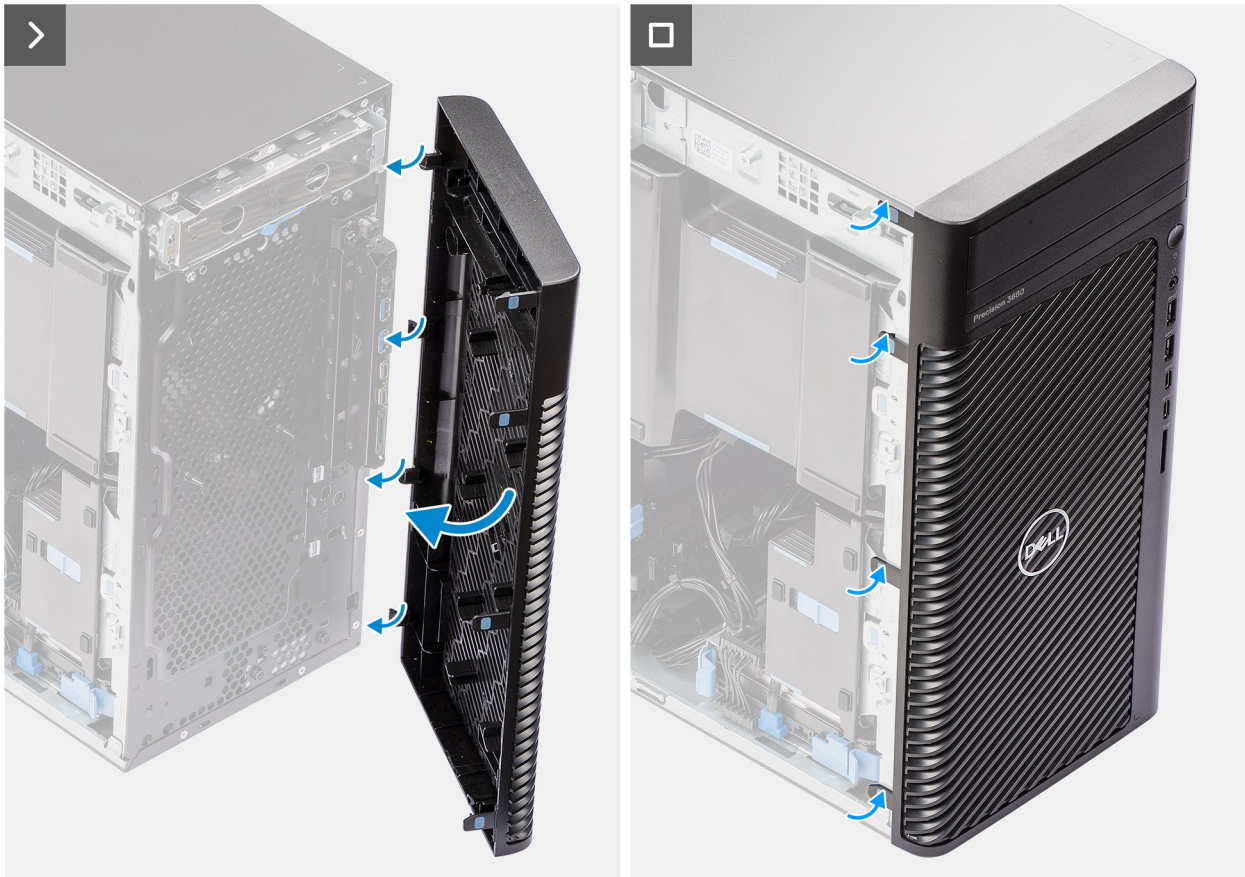
Figure 13. Installing the front bezel
