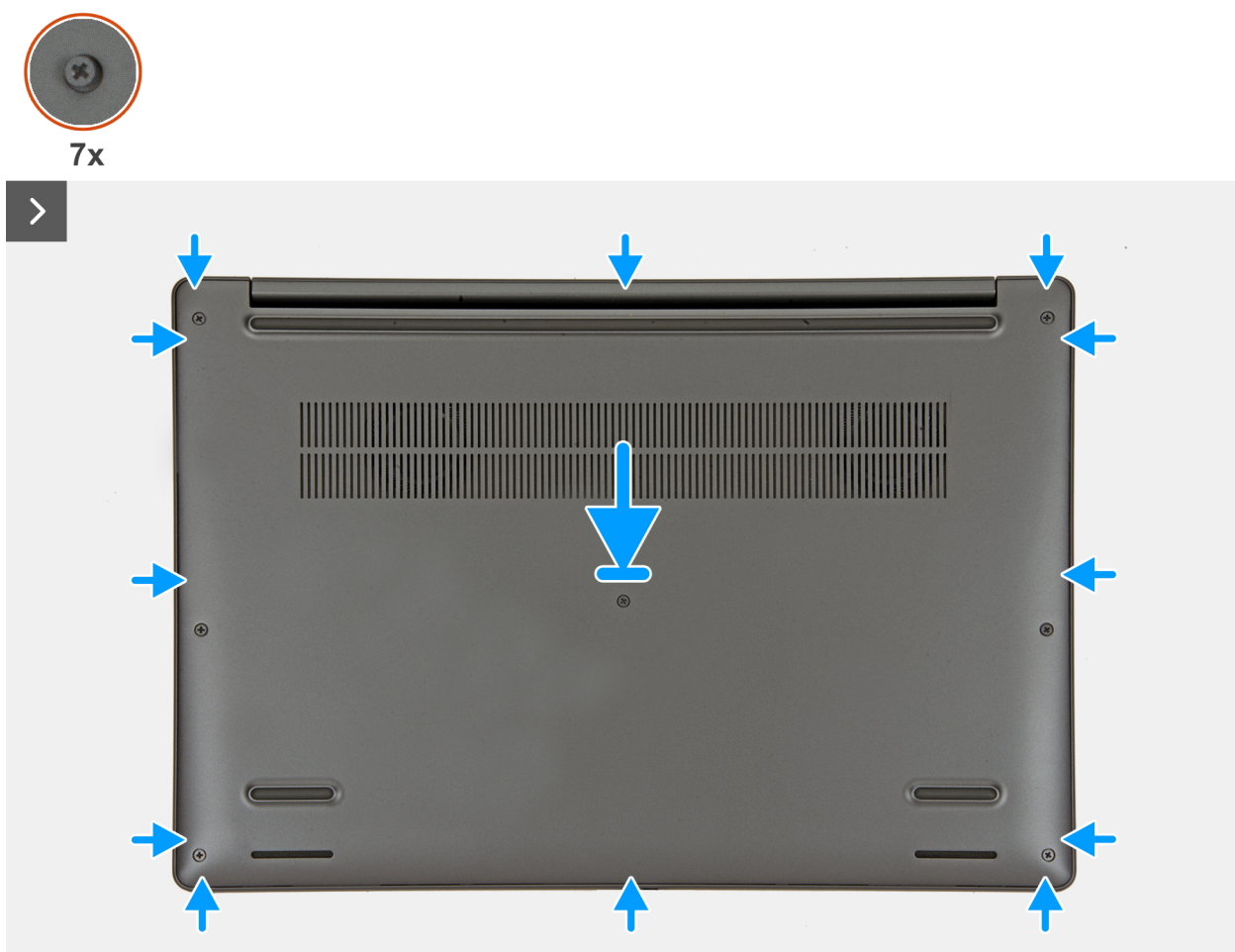
Figura 18. Installing the base cover
