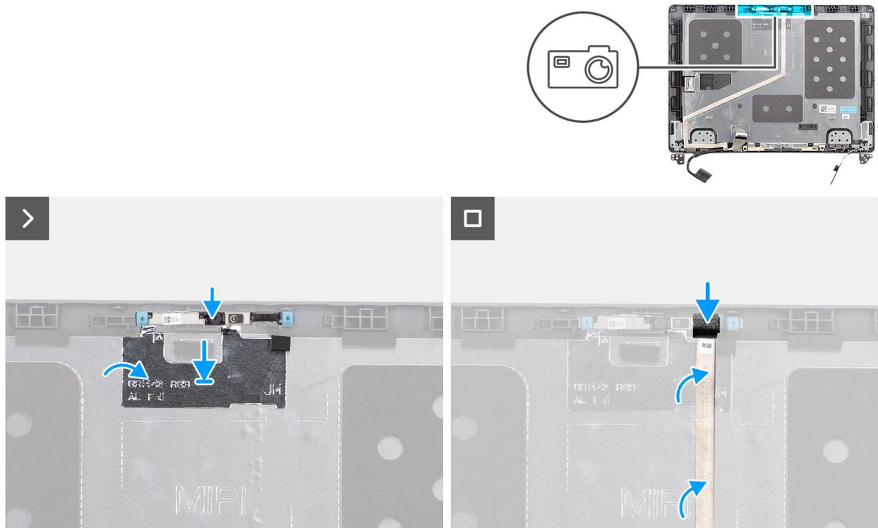
Figura 71. Installing the camera
