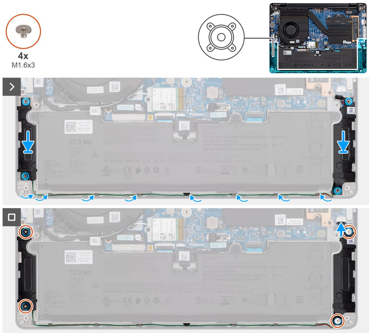
Figura 29. Installing the speakers
