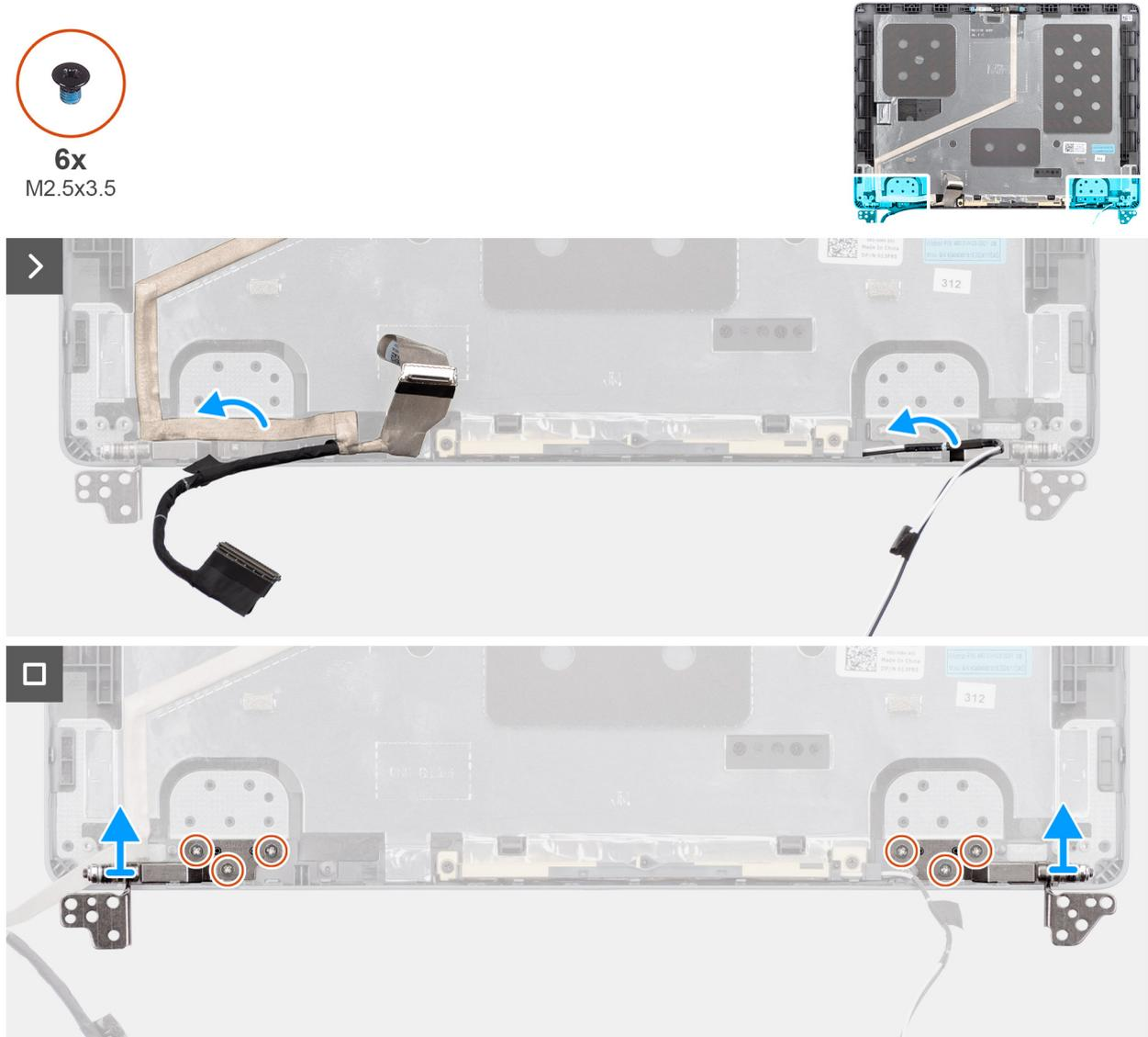
**Figura 66. Removing the display hinges**
