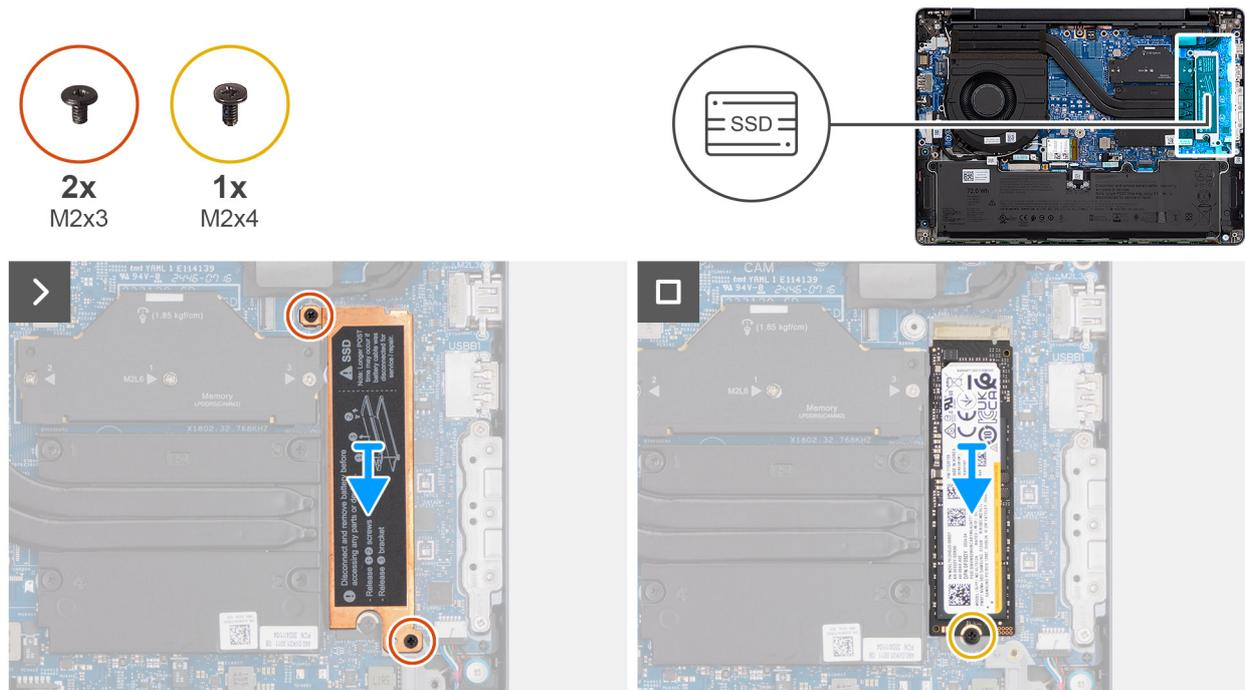
**Figura 24. Removing the M.2 2280 solid state drive**
