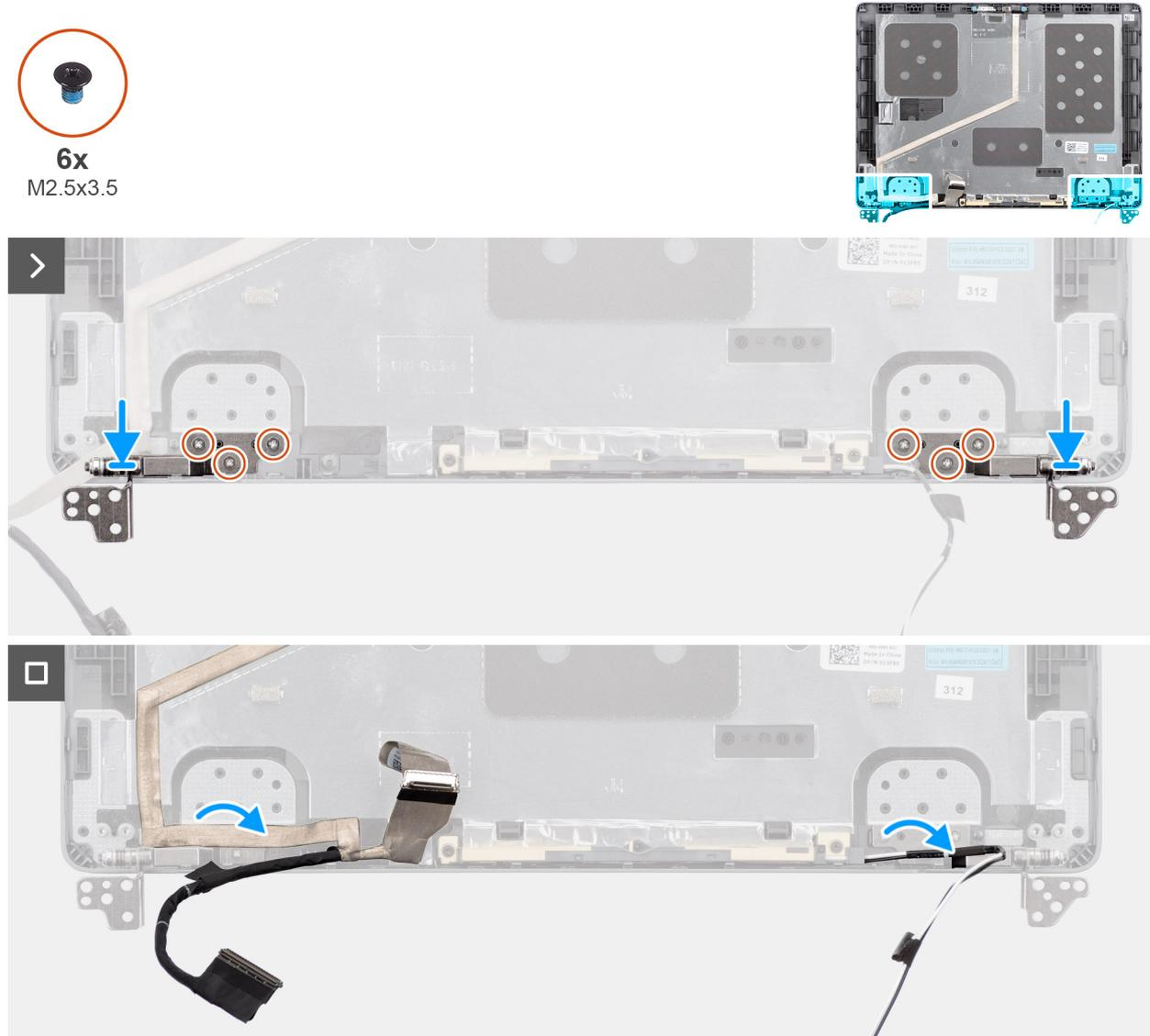
Figura 67. Installing the display hinges
