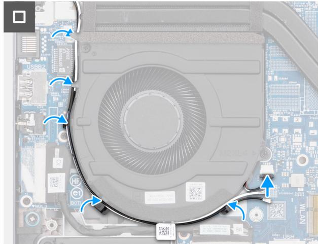
**Figura 32. Installing the fan**
