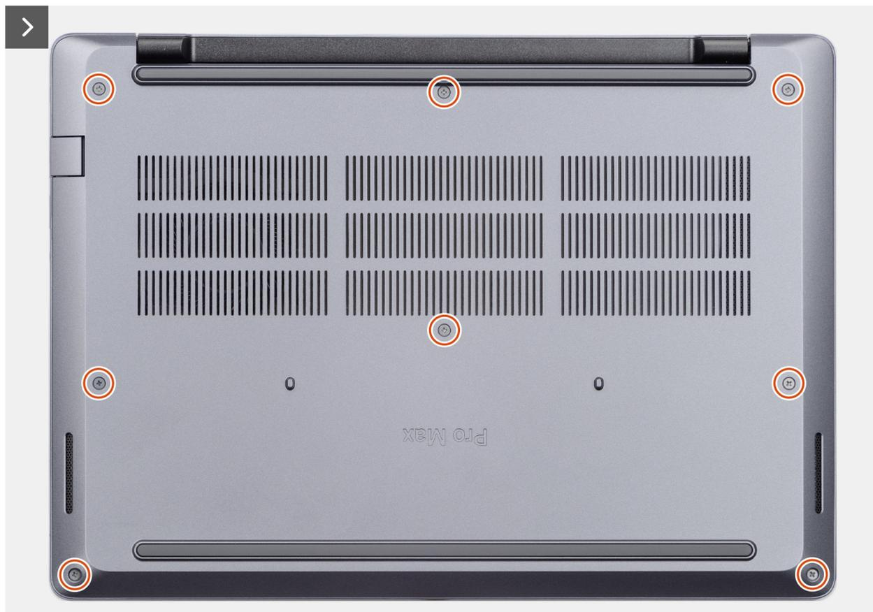
Figura 11. Removing the base cover
