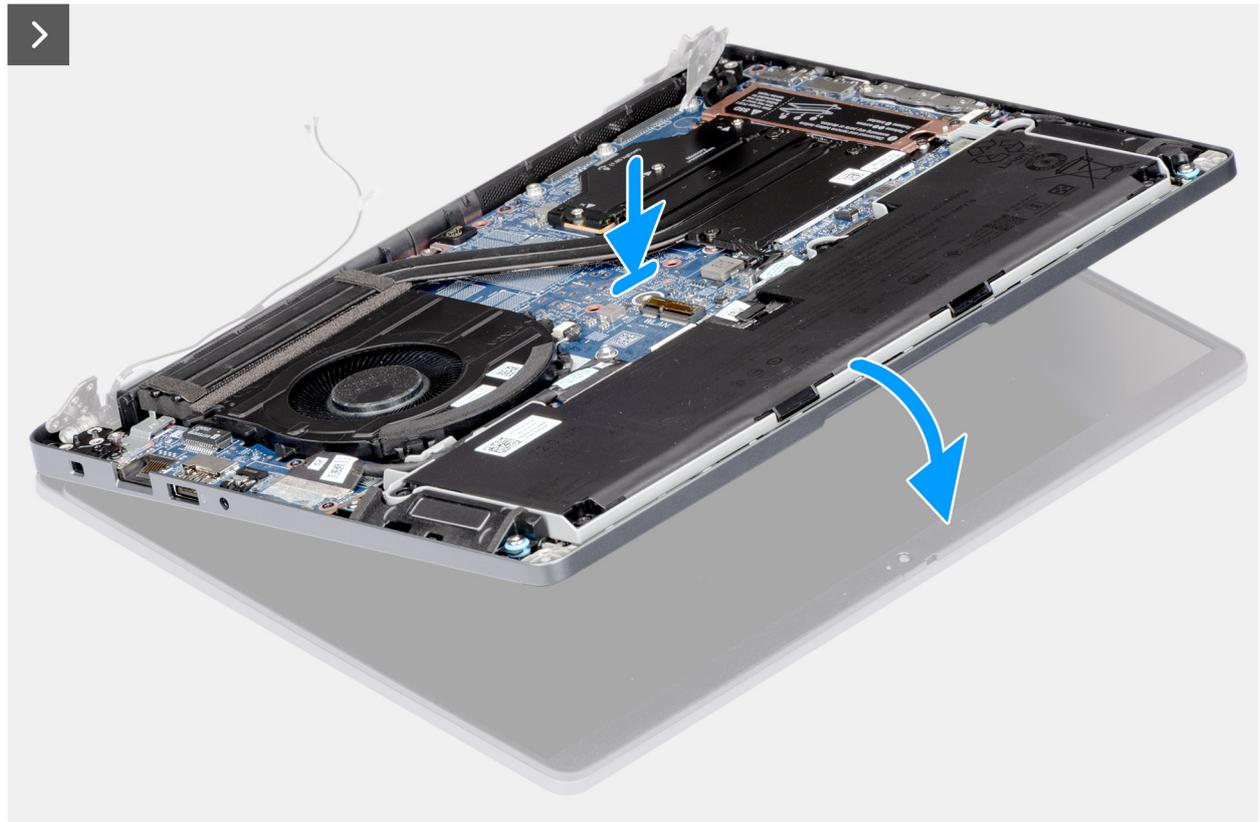
Figura 50. Installing the display assembly
