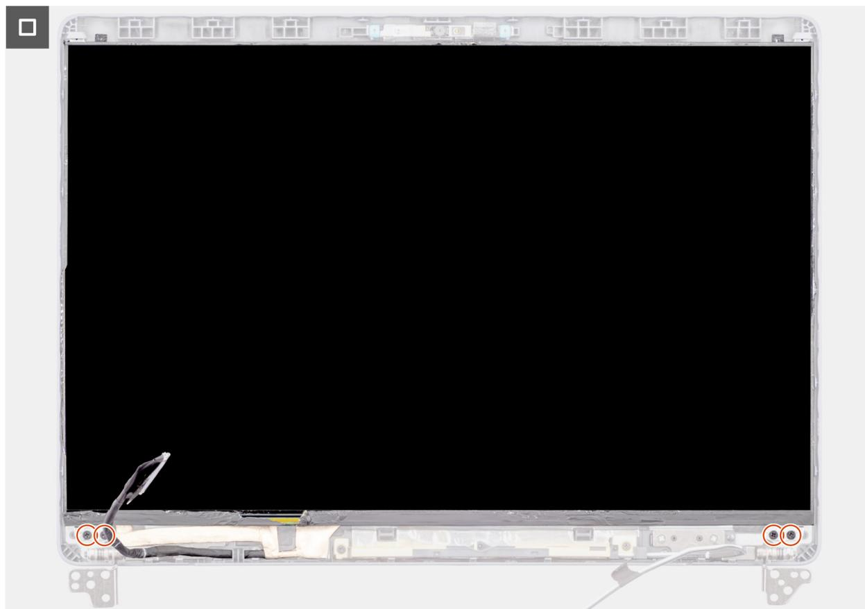
**Figura 65. Installing the display panel**
