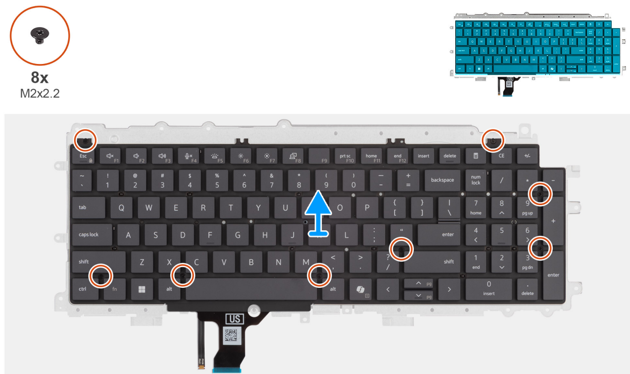
Figura 66. Removing the keyboard support plate
