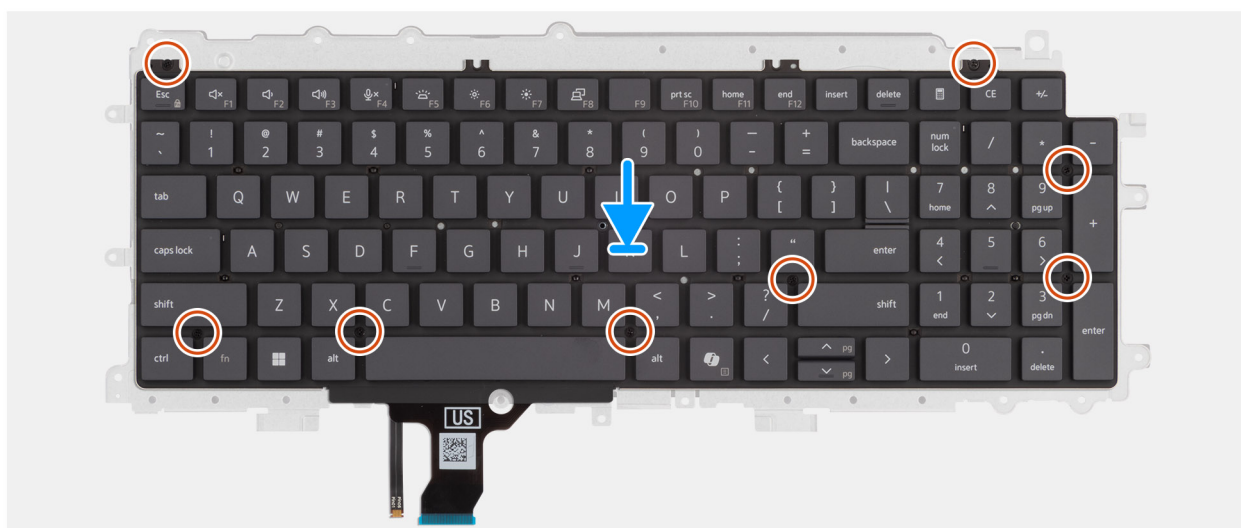
Figura 69. Installing the keyboard support plate
