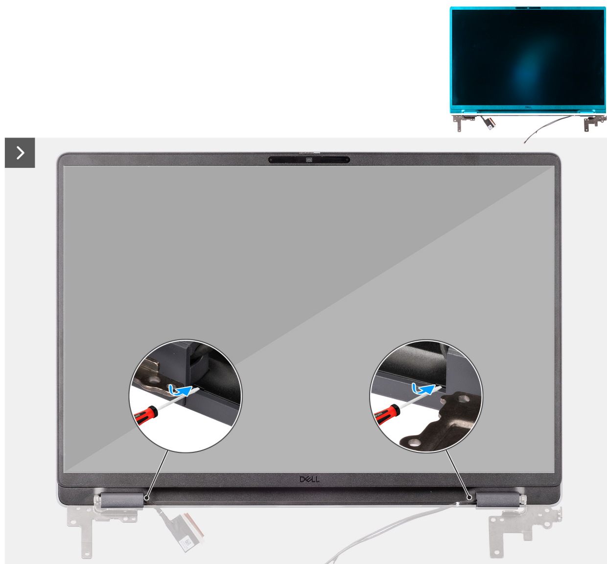
Figura 77. Removing the display bezel
