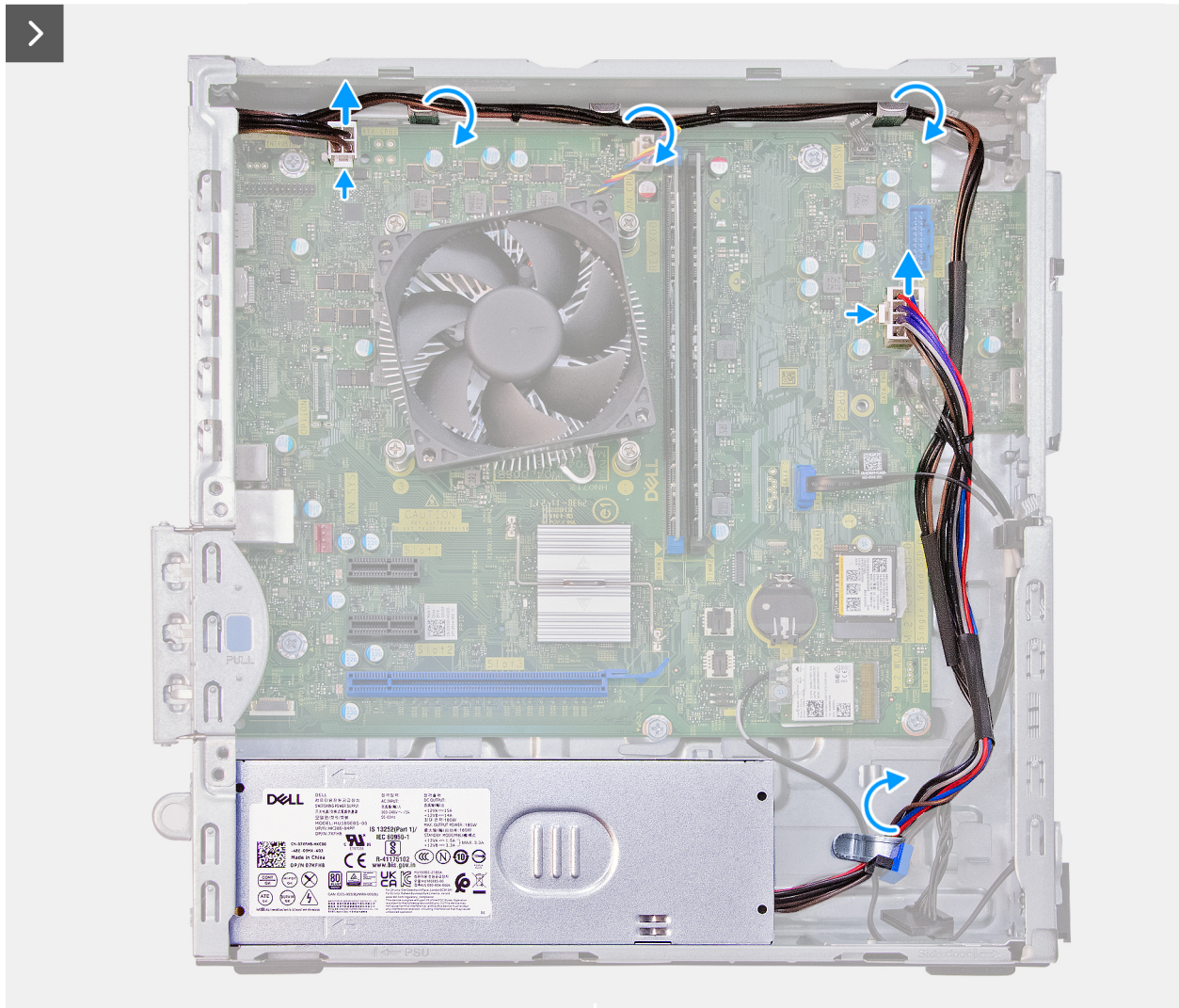
Figure 33. Removing the power-supply unit
