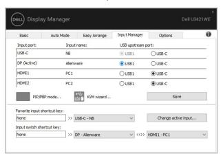
You can also use the **KVM wizard** to assign USB upstream ports to video inputs and select display partition for multiple devices.
