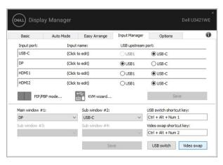
You can assign a USB upstream port with your video input. The assigned USB upstream port will be connected to the computer when its video is showing on the monitor.
