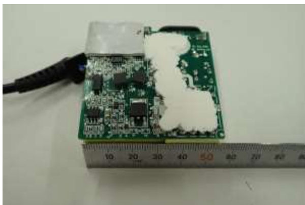
AC Adapter printed circuit board
