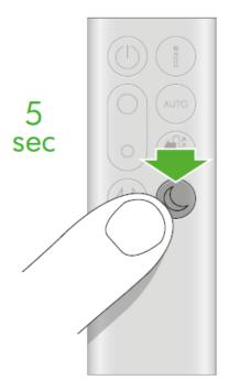
Pressing the night mode and sleep timer button on the bottom right of the remote
