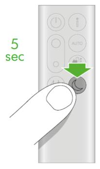
Pressing the night mode and sleep timer button on the bottom right of the remote
