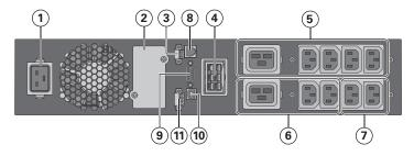
(\*) Primary and Grouped outlets (⑤), ⑥), ⑦) are protected by 20A circuit breakers.
