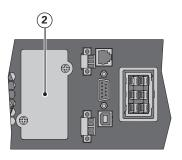
It is not necessary to shutdown the UPS before installing a communication card.
