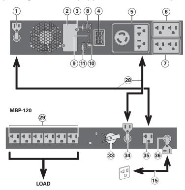
The **HotSwap MBP** module makes it possible to service or even replace the UPS without affecting the connected loads.
