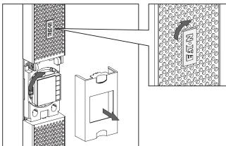
Adjustment of the angle of vision of the LCD panel.
