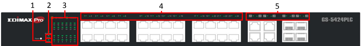
Figure 4 – GS-5424PLC Front View LED Indicators
