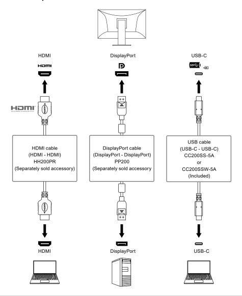
When two PCs are connected to one monitor, you can link the input signals with the USB ports to use a USB device connected to the monitor from both PCs by switching between them. For details, refer to "KVM" (page 26).
