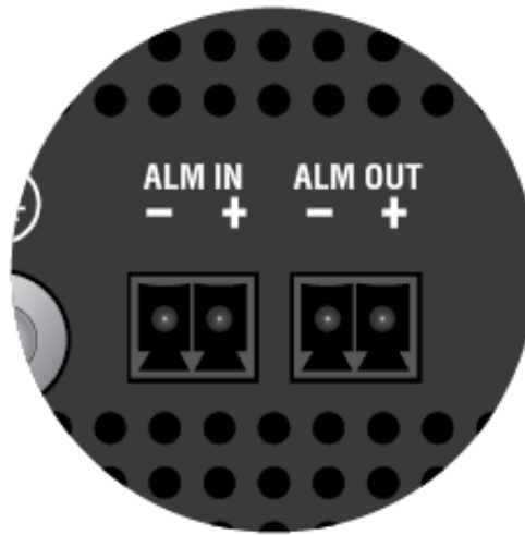
Figure 38. Polarity Legend for the Alarm Connectors
