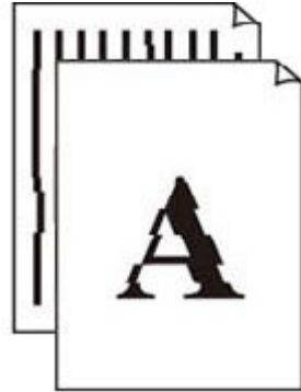
Lines Are Misaligned/Distorted
