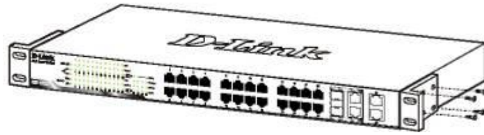
Figure 2.2 – Attach the mounting brackets to the Switch
