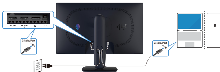
Figure 8. Connecting the DisplayPort (DP to DP) cable
