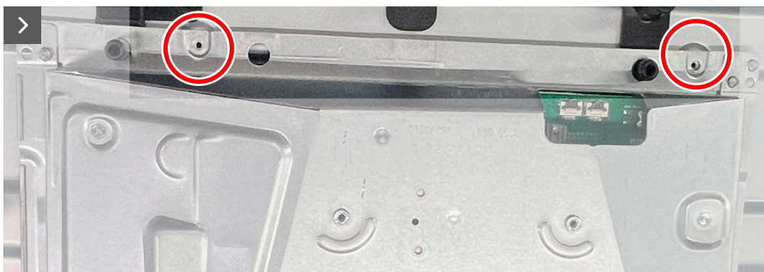
Figure 26. Installing the metal shield
