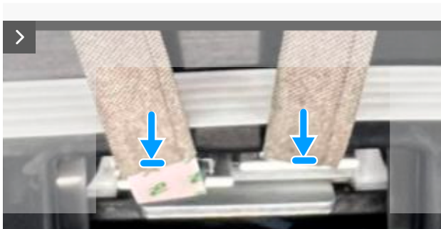
Figure 28. Installing the metal shield
