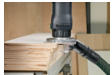
Chamfering plastic or solid wood veneer.
