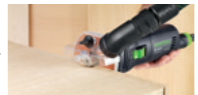
Flush trimming of plastic or solid wood veneer.
