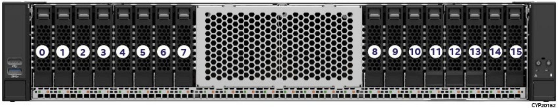
Figure 25. 2U 16 x 2.5" Front Drive Bay Configuration
