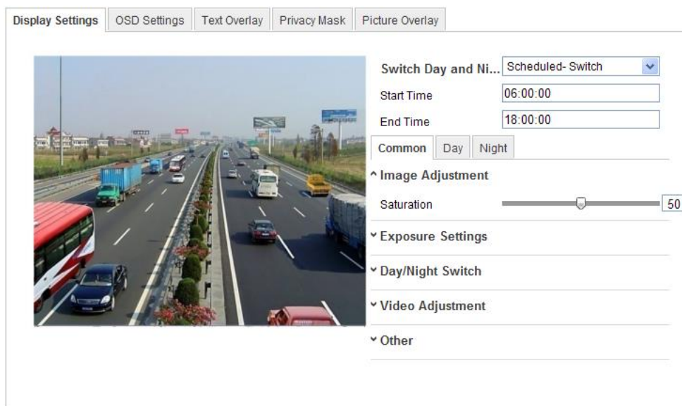
Figure 6-35 Day/Night Scheduled-Switch Configuration Interface
