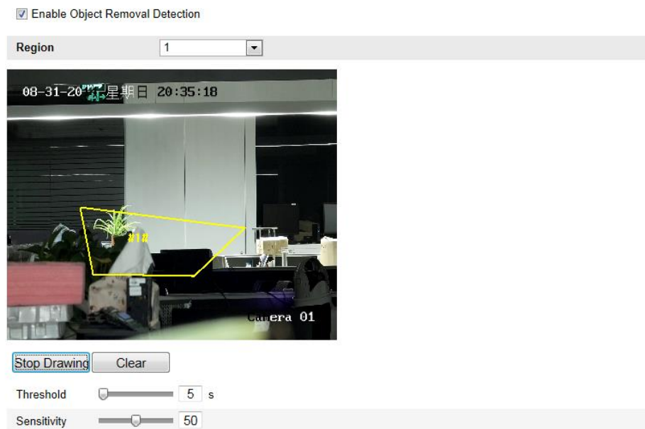
Figure 6-65 Configuring Object Removal Detection
