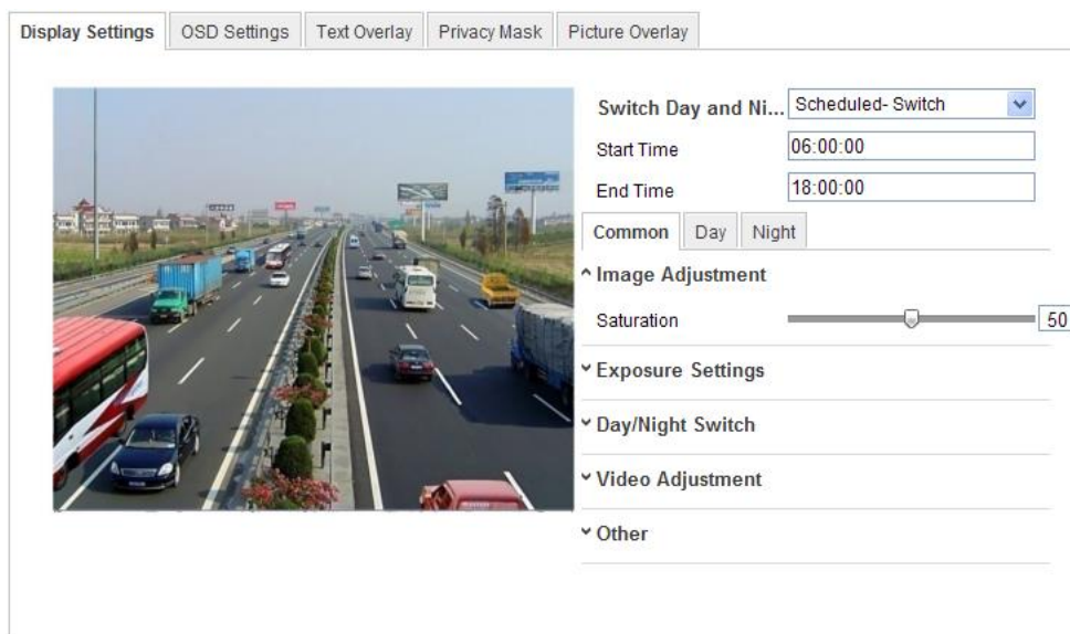
Figure 6-35 Day/Night Scheduled-Switch Configuration Interface
