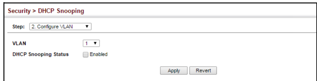
Figure 192: Configuring DHCP Snooping on a VLAN
