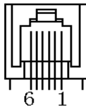
Fig.6.7-1 Schematic drawing of cash drawer interface
