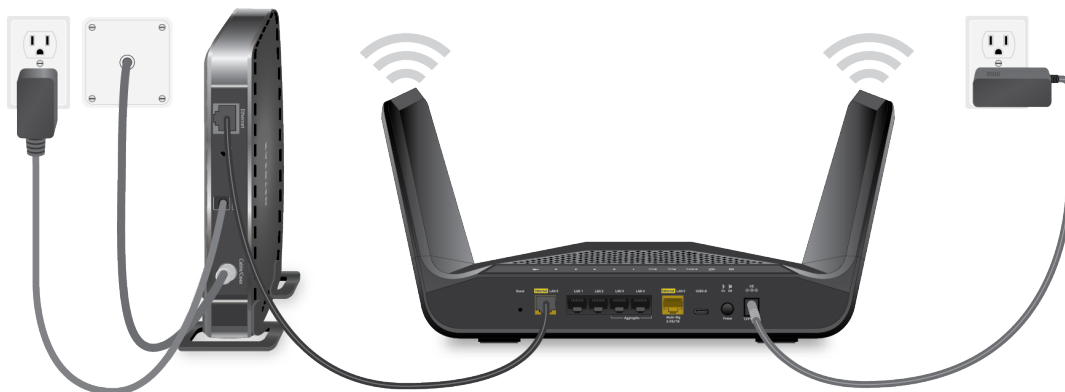
Figure 6. Router connected to a modem
