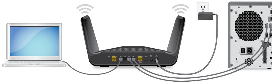
Figure 8. Ethernet port aggregation to a LAN device
