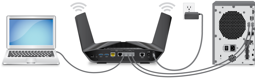
Figure 9. Ethernet port aggregation to a LAN device
