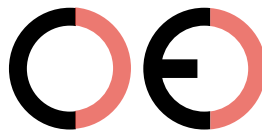
False CE Mark (too far)
