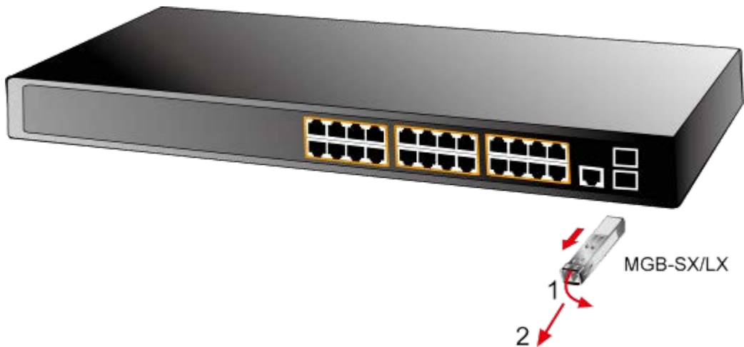
Figure 2-1-13: How to Pull Out the SFP Transceiver
