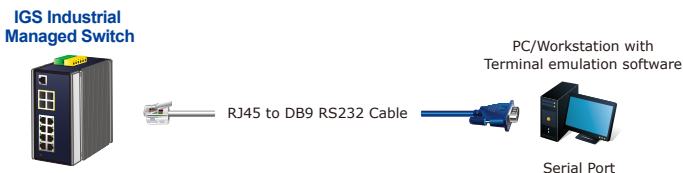
Figure 4-1: Industrial L2+ Managed Switch Console Connectivity
