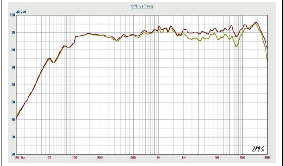
Frequency Response Graph: (dB SPL vs Frequency)
