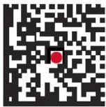
Figure 3-9 DS36X8-DP and DS36X8-DPA Aiming Pattern
