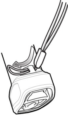
Figure 1-20 Insert Lanyard Loop
