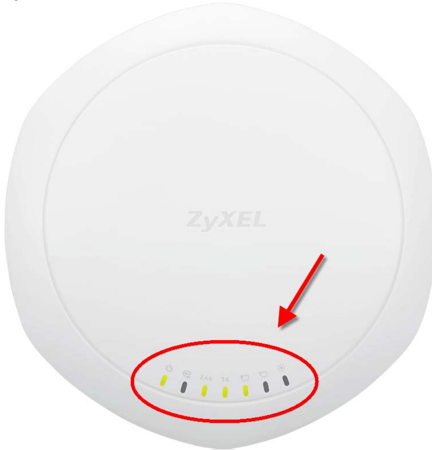
Figure 18 NWA1123-AC PRO LEDs
