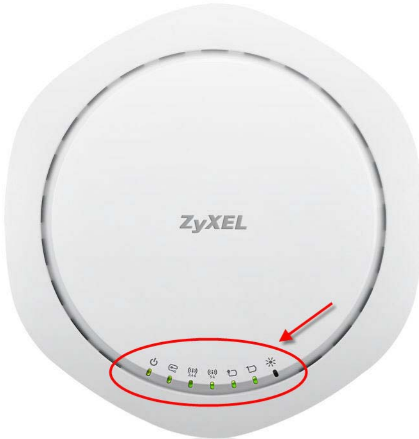
Figure 20 WAC6502D-E, WAC6502D-S, or WAC6503D-S LEDs
