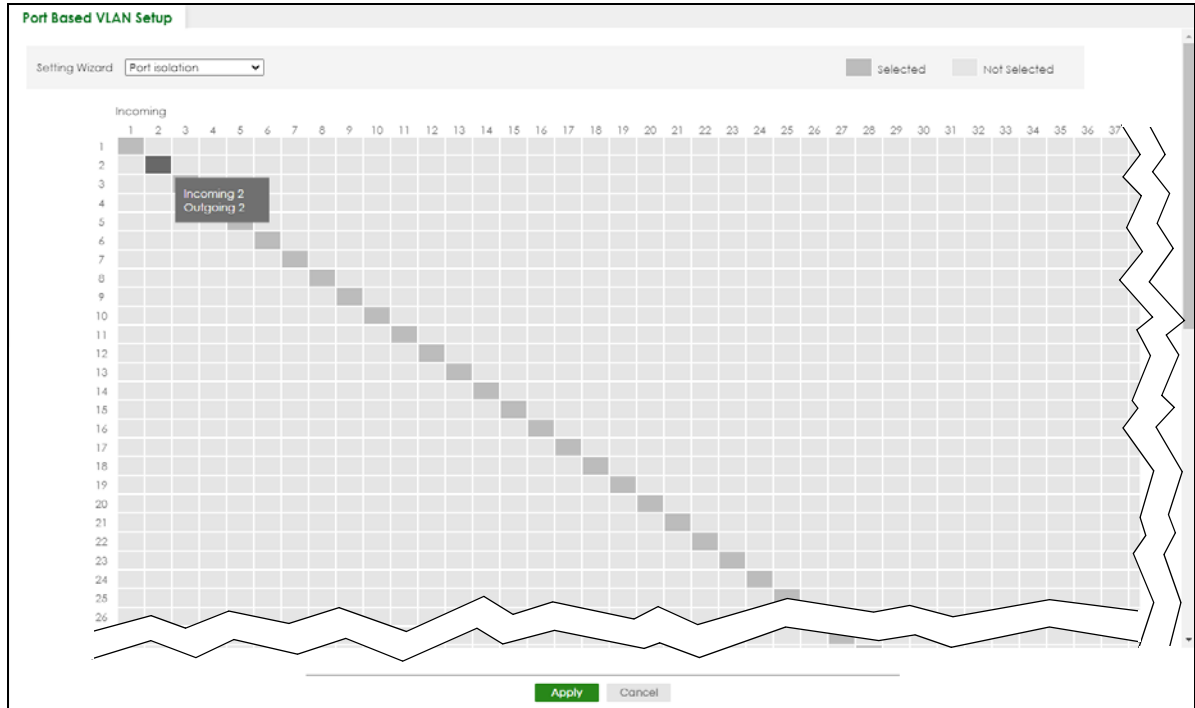
Figure 288 SWITCHING > VLAN: Port Based VLAN Setup (Port Isolation)
