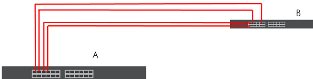
Figure 160 Trunking Example – Physical Connections
