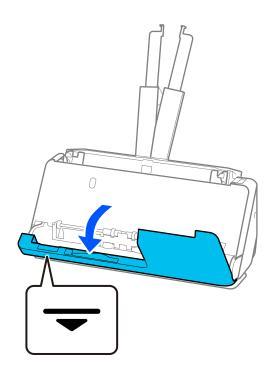
3. Pull the lever to open the scanner cover.
