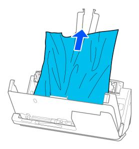
5. If you cannot pull originals straight up, carefully pull out any jammed originals from the output tray in the direction of the arrow.
