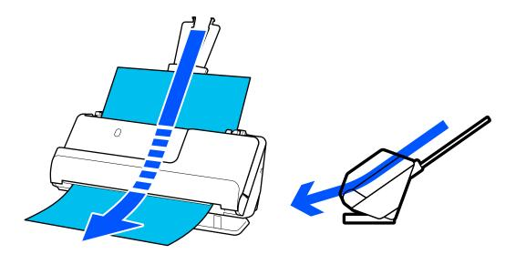
When the scanner is changed to the straight path position, the <u>U</u> light on the control panel turns on.
