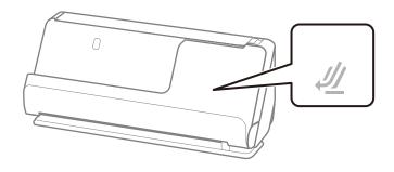
$\Box$  When scanning award certificates and other thick originals (originals with a thickness 127 g/m<sup>2</sup> or more), scan in the straight path position and load only one original at a time.
