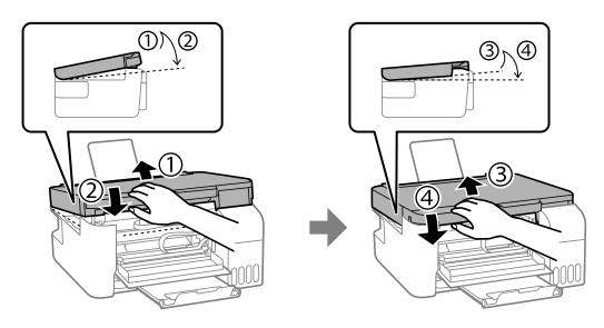
*Note: The scanner unit must be closed completely before it can be opened again.*
