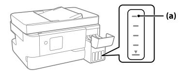
8. Align the top of the ink bottle with the filling port, and then insert it straight into the port to fill ink until it stops automatically at the upper line.
