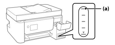
8. Align the top of the ink bottle with the filling port, and then insert it straight into the port to fill ink until it stops automatically at the upper line.
