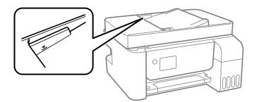
The original slips when paper dust adheres to the roller.
