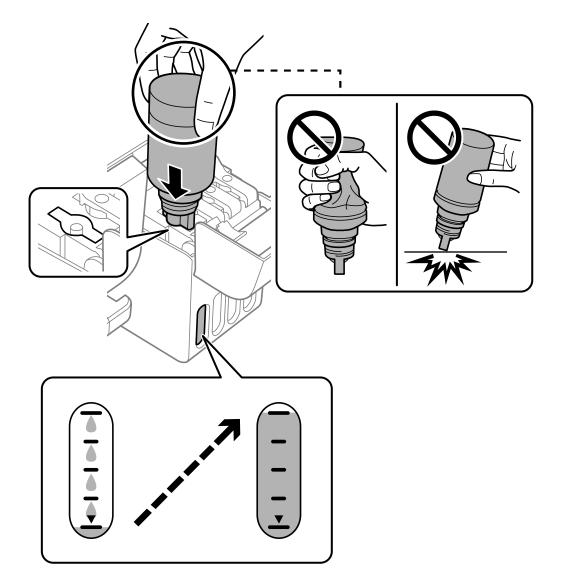
If the ink does not start flowing into the tank, remove the ink bottle and reinsert it. However, do not remove and reinsert the ink bottle when the ink has reached the upper line; otherwise ink may leak.
