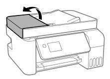
2. Use a soft, moist cloth to clean the roller and the interior of the ADF.
