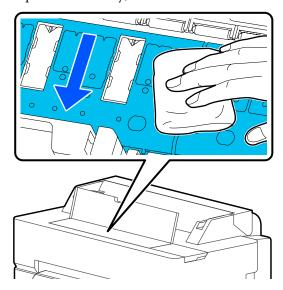
If any paper particles (resemble white powder) have accumulated in the holes shown in the illustration below, use a pointed object such as a toothpick to push them in.
