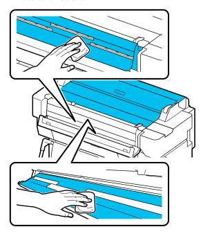
Use the cleaning kit, or the clean side of the soft cloth, to thoroughly wipe the area shown in blue in the illustration below.
