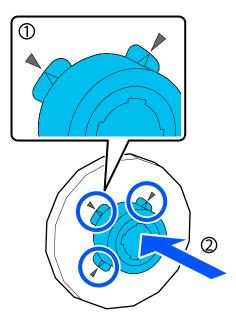
Place the roll paper on a flat surface and then insert the spindle.
