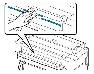
Use the cleaning kit, or the clean side of the soft cloth, to wipe the glass surface.
