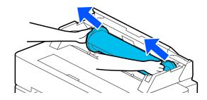
Detach the transparent flange from the spindle.
