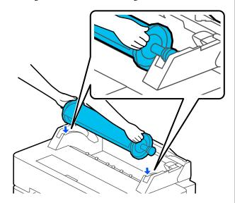
Slide the spindle in along the rails, and set the spindle's both ends in the spindle holders.
