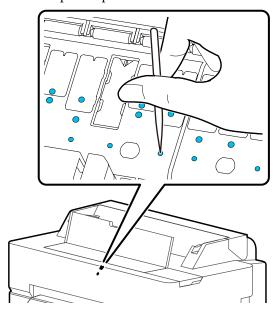
Remove paper particles and dust around the outer edges with commercially available cotton swabs.
