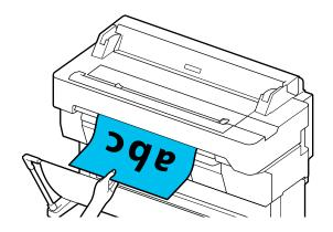
Printing starts when the original has been completely removed.
