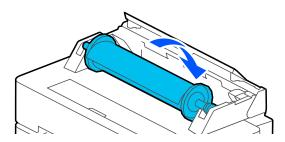
10 Check that the leading edge of the roll paper is not bent and then insert it into the paper slot until you hear a beep.
