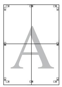
After joining all the sheets, trim off the borders by cutting along the cut guides (outside the X marks).
