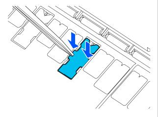
Gently press the pad for borderless printing until it is seated flatly in place.
