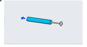
Attach the transparent media edge guide to the spindle.
