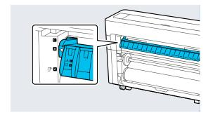
Raise the spindle lock lever for roll1.
