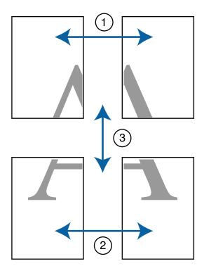
Ready the two top sheets and trim the excess from the left sheet by cutting along the line joining the two join guides (the centers of the X marks).
