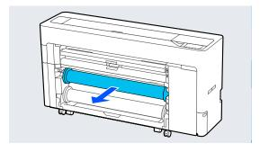
Remove the transparent media edge guide from the spindle.
