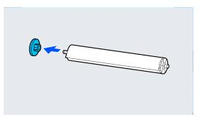
Remove the roll paper that has been taken-up from the spindle.
