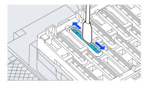
(3) Hold the cleaning stick so that it is vertical, and wipe the outer areas of all of the capping stations.
