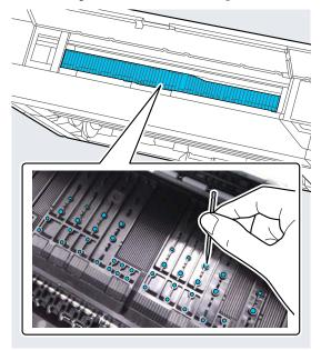
The reverse side of the printed paper is soiled, use a cleaning stick to wipe the area shown below from the back to the front.
