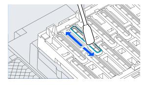
(5) Hold the cleaning stick so that it is vertical, and wipe the guides of all of the capping stations.
