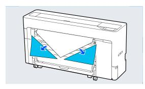
Check the take-up direction and attach the end of the paper to the roll core.
