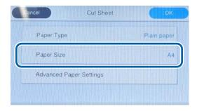
If the loaded paper does not match the paper size displayed on the screen, press **Paper Size** to set the paper size.
