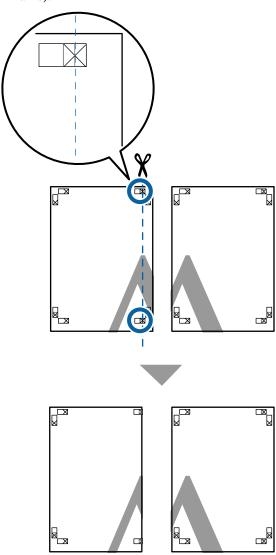
Lay the upper left sheet on top of upper right sheet. Lineup the X marks as shown in the illustration below, and temporarily fasten them using an adhesive tape on the back.
