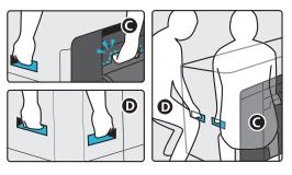
☐ Do not tilt the product more than 10 degrees forward or back while moving it. Failure to observe this precaution could cause the product to tip over or ink to leak.
