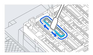
(4) Wipe the edges of all of the capping stations with the flat surface of the cleaning stick.
