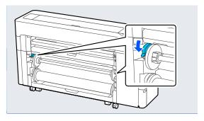
Press the pause/resume button, and then use the take-up direction switch to select either printed side in or printed side out.
