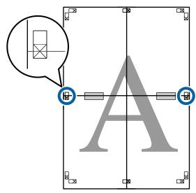
With the two sheets overlapping, trim the excess by cutting along the line joining the two cut guides (the lines above the X marks).
