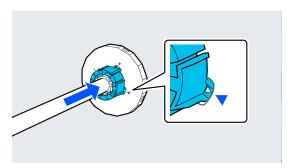
Insert the spindle with the roll paper facing the direction shown in the illustration.
