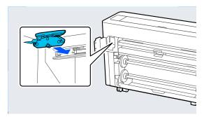
7 Tighten the screw that secures the cutter with the cross-head screwdriver.
