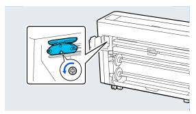
Remove the old auto cutter blade from the printer.
