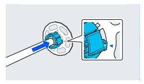
Insert the spindle into the roll core.
