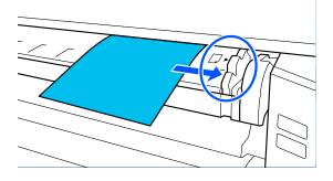
Insert the paper straight into the printer to the position shown in the illustration.
