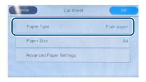
If the paper type displayed does not match the paper type that you have loaded, press **Paper Type** to set the paper type.
