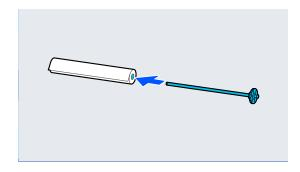
Attach the transparent media edge guide to the spindle.
