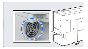
If the printer is particularly dirty, dampen the cloth with water containing a small amount of neutral detergent, and then firmly wring the cloth dry before using it to wipe the printer's surface. Next, use a dry cloth to wipe away any remaining moisture.
