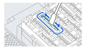
(2) Hold the cleaning stick so that it is vertical, and wipe the inner areas of all of the capping stations.
