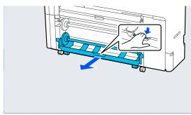
Remove the spindle.
