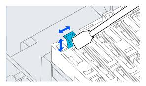
(6) If there is any fluff or dust in the caps, remove it with the tip of the cleaning stick or with tweezers.
