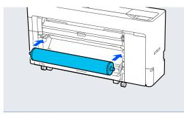
10 Lower the spindle lock lever.
