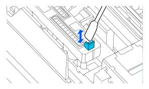
(4) If there is any fluff or dust in the caps, remove it with the tip of the cleaning stick or with tweezers.
