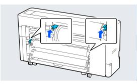
Remove the spindle.
