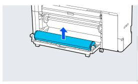
Remove the transparent media edge guide from the spindle.
