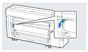
Remove the spindle.
