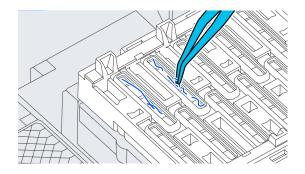
Use a new cleaning stick to wipe any dirt off the wiper.
