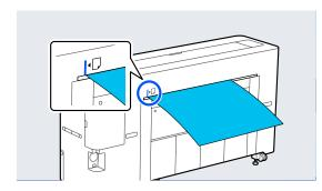
Insert the paper straight into the printer to the position shown in the illustration.
