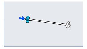
Place the spindle into the grooves with the black media edge guide on the right.
