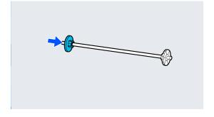
Place the spindle into the grooves with the black media edge guide on the right.
