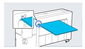
Insert the paper straight into the printer to the position shown in the illustration.
