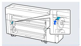
A Remove the spindle.
