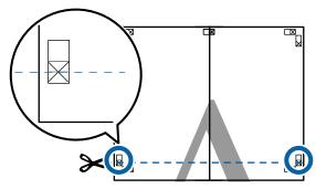
Lay the upper sheet on top of the lower sheet. Lineup the X marks as shown in the illustration below, and temporarily fasten them using an adhesive tape on the back.
