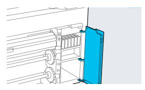
Place your finger into the gap and remove the ink cartridge.
