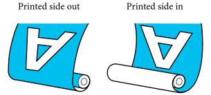
Taking-up with printed side out places the printed surface on the outside of the roll.
