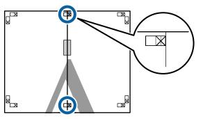
With the two sheets overlapping, trim the excess by cutting along the line joining the two cut guides (the lines to the left of the X marks).
