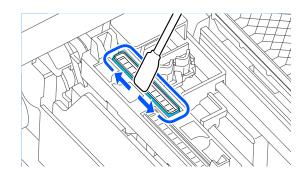
(2) Wipe the edges of all of the suction caps with the flat surface of the cleaning stick.
