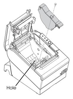
3. Tighten the enclosed screw to fix the roll paper guide.
