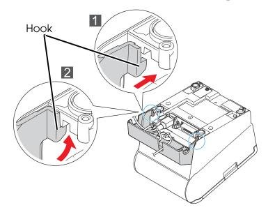
To remove the connector cover, turn the printer over, and push the connector cover down while pushing both sides of the connector cover inward to detach the hooks from the printer case.
