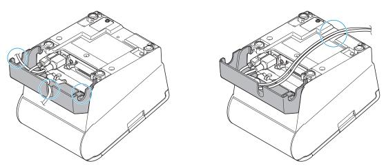
If you want to pass the USB cable through the cable exit on the back, fit the cable under the hook on the printer to prevent the cable from coming off.
