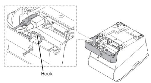
After the cable arrangement, turn over the printer, and make sure the cables are not pinched.
